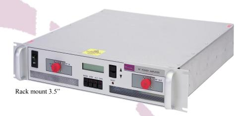
These linear amplifiers are only 3.5 inches high and control interface options include IEEE/RS232 and Ethernet connectivity.
