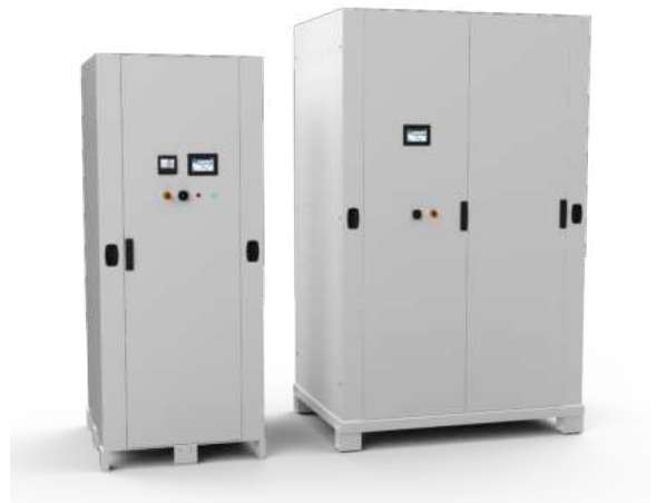
Figure 10: REGATRON's liquid-cooled system solutions up to IP54 with various power levels, e.g. 54...162 kW (left) and 216...324 kW (right). The remote control unit RCU, indicator lights, emergency stop button, and main switch allow the user to operate the system on the enclosure's front door.
