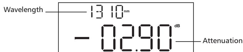
**Note:** *The attenuation value is the actual insertion loss between the input and output ports including connectors.*
