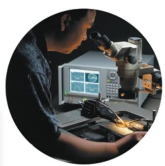
Use TRL calibration for accurate in-fixture or on-wafer measurements.
