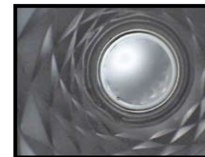
Image with WiDER™ gain applied. WiDER™ gain brightens the darker areas while maintaining the light level and details shown in the bright area.
