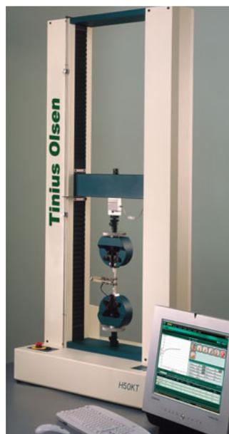
**Fig 37.** Model H50kT with HT21 grips
