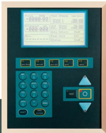
The single column materials testing machines have frame capacities of 1 kN or 5 kN (200 lbf or 1,000 lbf) and include two model types — the S series and the T series. These machines are designed to test a wide range of materials, including, but not limited to: plastics, films, paper, packaging materials, filter material, adhesives, foils, food, toys, medical devices and components, in tension, compression, flexure, shear, and peel.
