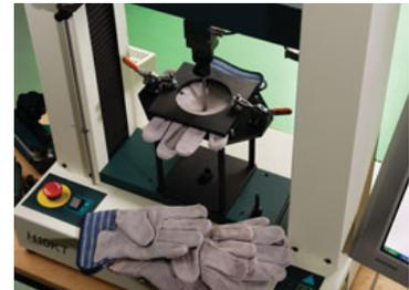
**Fig 30.** Testing the puncture resistance of work gloves
