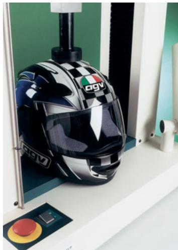
**Fig 27.** Compression test on crash helmet
