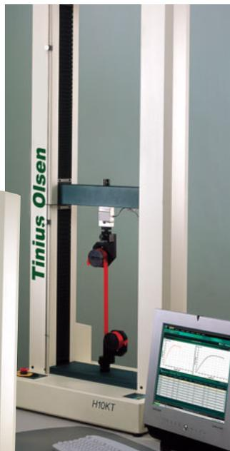
**Fig 35.** Model H10kT being used with HT29 grips to test thin rope
