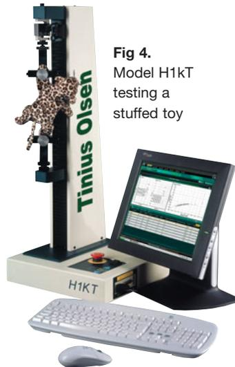
Fig 4. Model H1kT testing a stuffed toy
