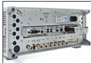
Figure 12. Data sanitization with removable hard drives in the X-Series signal analyzers
