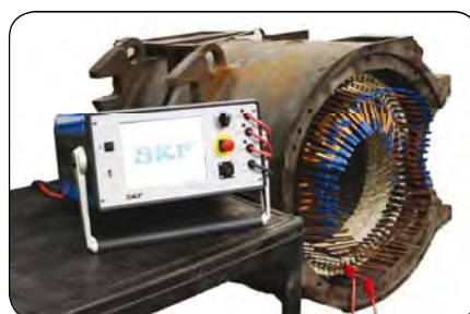
Testing individual coils within the stator.
