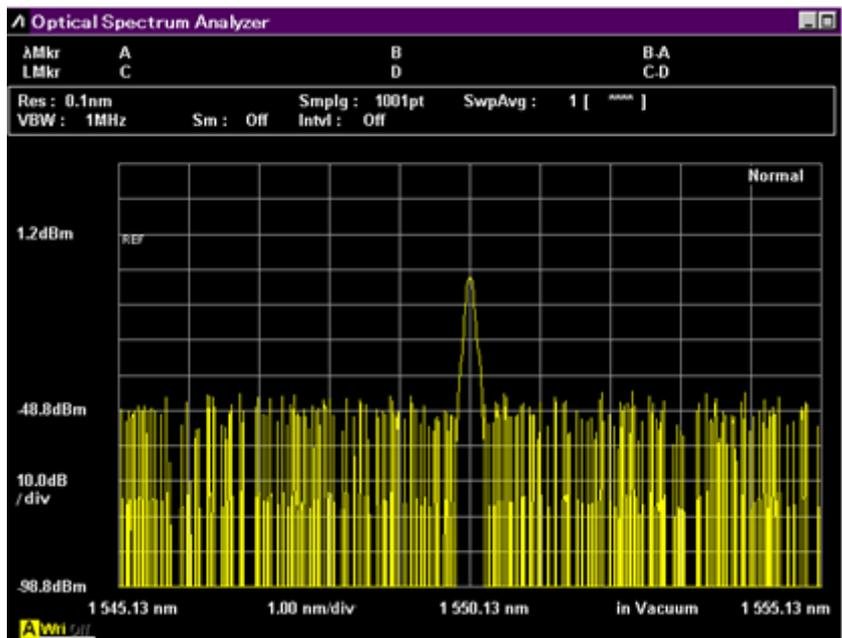
Figure 1.3-1 Example of Measurement at VBW 1 MHz
