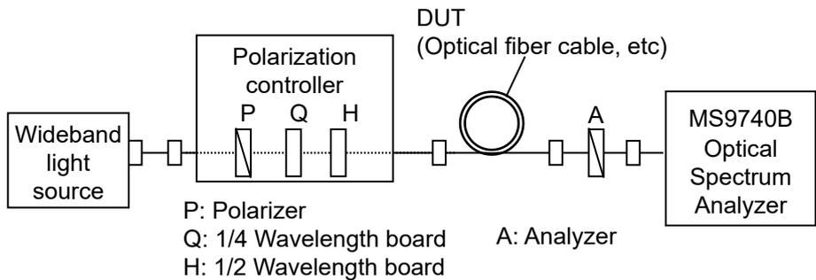
Figure 5.4.2-1 PMD Measurement System
