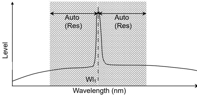
Figure 5.8.4-2 Integration Range for Only One Signal
