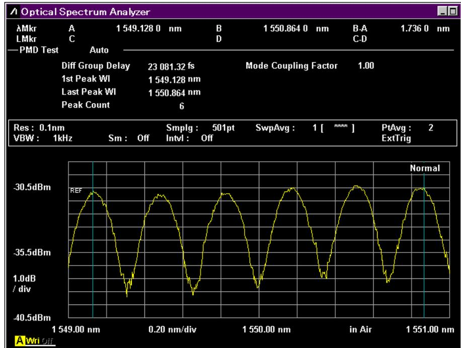
Figure 5.4-2 PMD-Test Example
