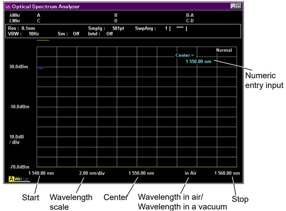
Figure 4.1-1 Names of Wavelength Display
