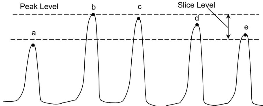
Figure 5.5.2-2 WDM Analysis Target Peaks
