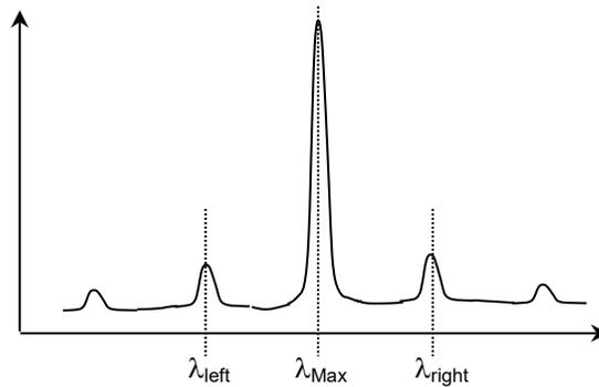
Figure 5.1.2-1 Position of Peak Wavelength and Side Mode
