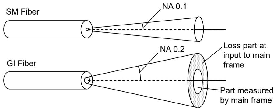
Figure 2.7-1 Difference in light radiated from optical fibers
