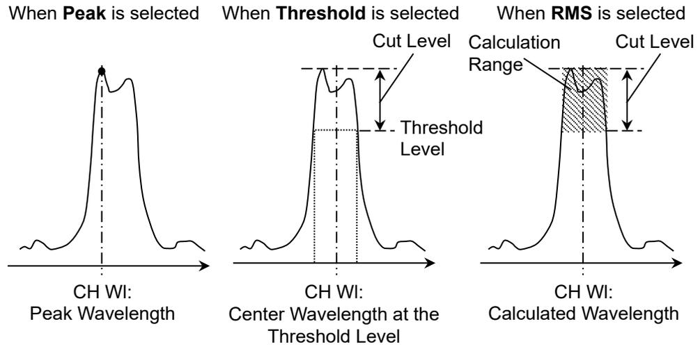
**Figure 5.9.3-3 Measurement Method for Signal Wavelength**
