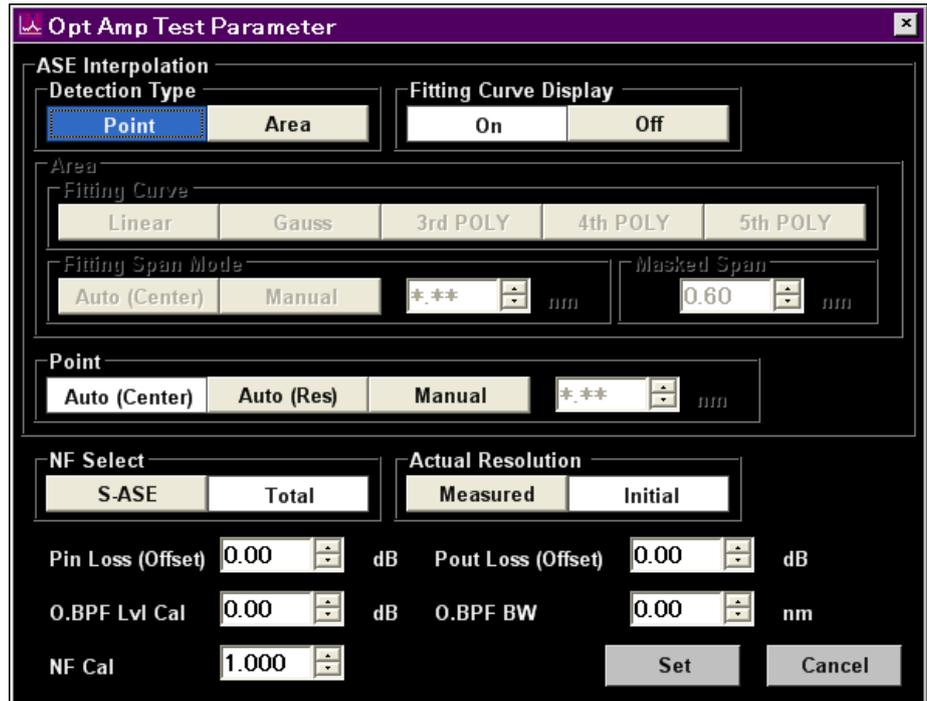
Figure 5.8.3-1 Opt Amp Test Parameter Dialog Box
