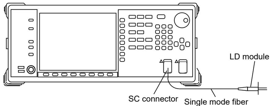
**Figure 3.2-2 Connection Example of Laser Diode Module**
