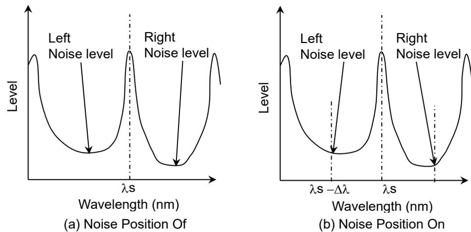
**Figure 5.5.3-3 Measurement of Noise at Noise Position**
