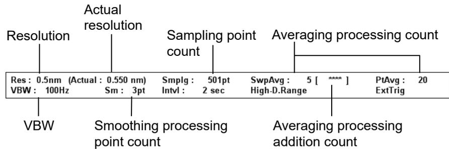
Figure 4.3-1 Measurement Condition Display Field
