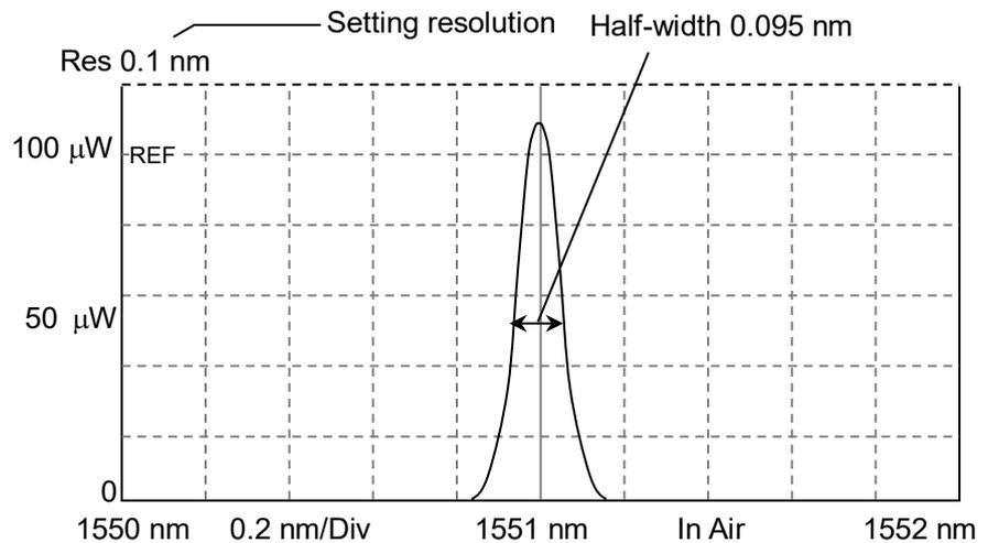
Figure 1.3-5 Measurement Example of Resolution 0.1 nm
