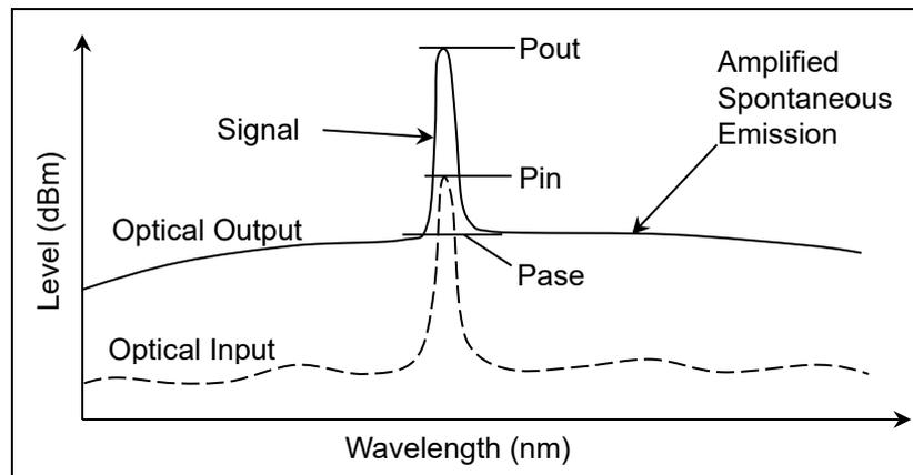
**Figure 5.7.1-1 Level Measured with Optical Amplifier Measurement Function**
