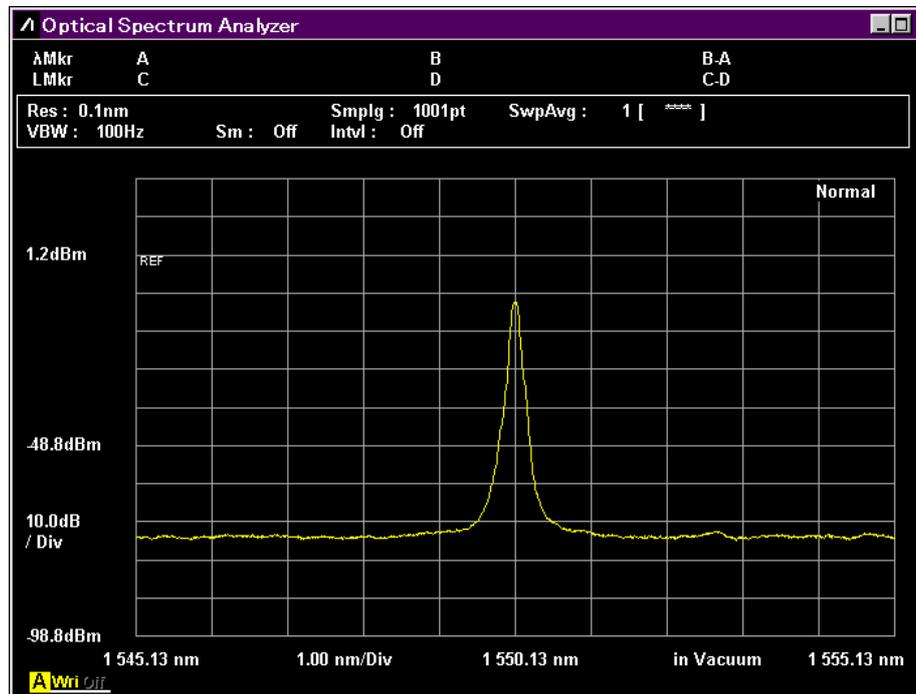
Figure 1.3-3 Example of Measurement at VBW 100Hz
