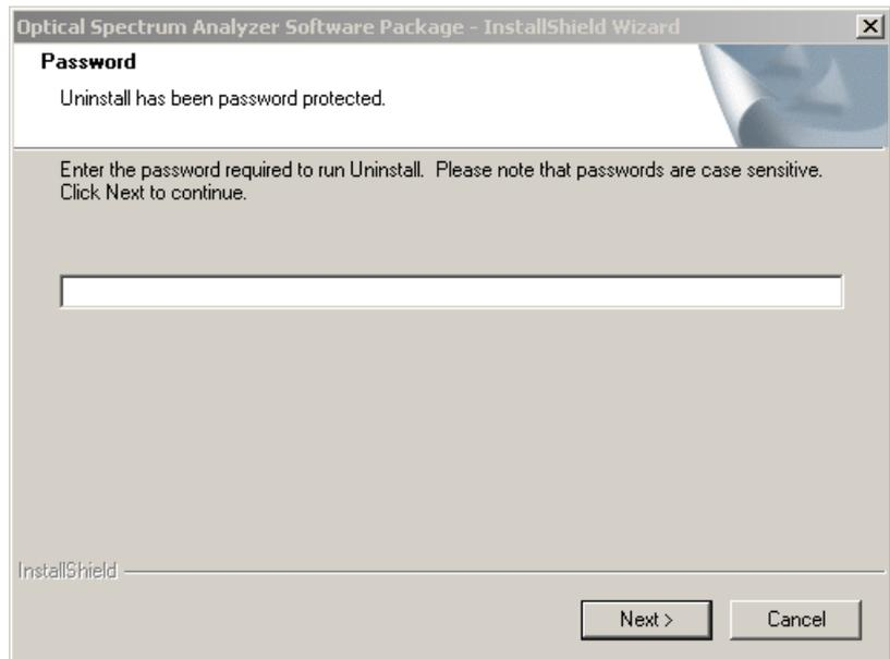
2. When installation is continued, enter “ms9740a\_osa” using the key board. Select **Next** using the key board or mouse and press **Enter**.
