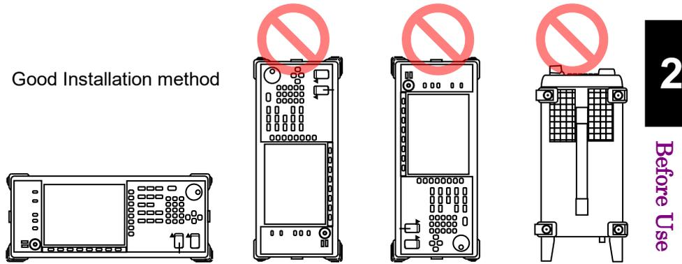
Figure 2.1.2-1 Installation Orientation
