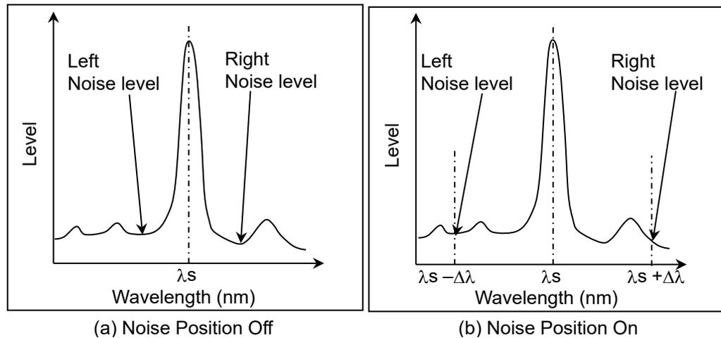
**Figure 5.6.2-3 Measurement of Noise at Noise Position**
