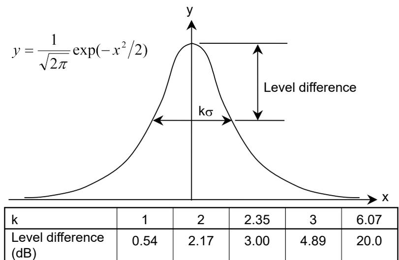
Figure 4.5.5-2 Multiplier k and Gaussian Distribution Function Level Difference
