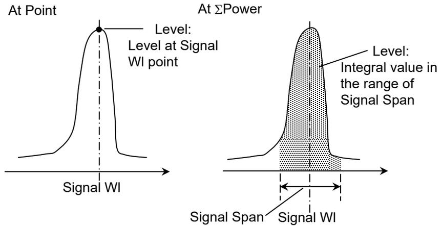
Figure 5.5.2-4 Measurement Method for Signal Level
