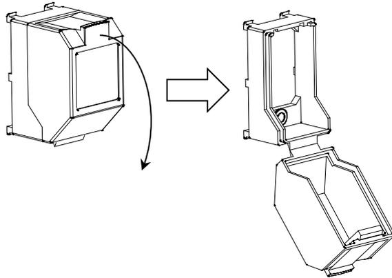
Figure 2.2.1-2 How to Opening the Optical Connector Cover
