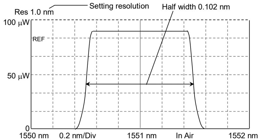
Figure 1.3-7 Measurement Example of Resolution 1.0 nm
