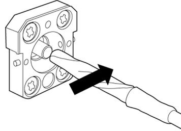
Figure 7.4-3 Cleaning the Ferrule End Surface 3
