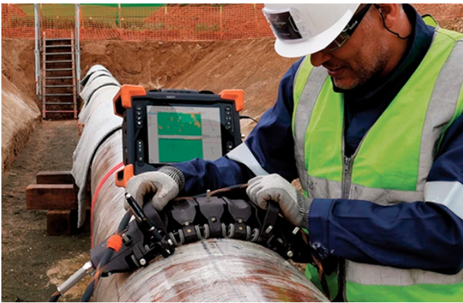
Figure 4: Ditch pipeline inspection using Sypne™ paired with Reddy.
