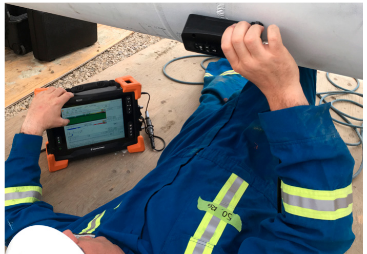
Figure 2: Detecting and sizing cracks in carbon steel welds using the Sharck™ paired with Reddy.
