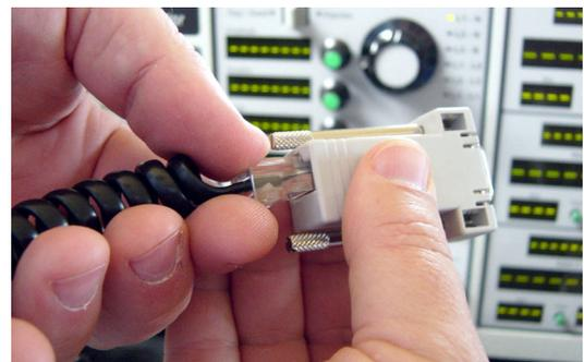
*Connect one end of the coms cable to the IPC PC Port on your IPC's front panel, near the power switch. Connect the other end to the serial port on your computer using the 9-pin adaptor supplied. If your computer lacks a serial port, use a USB-to-serial adaptor (use Belkin model F5U103).*
