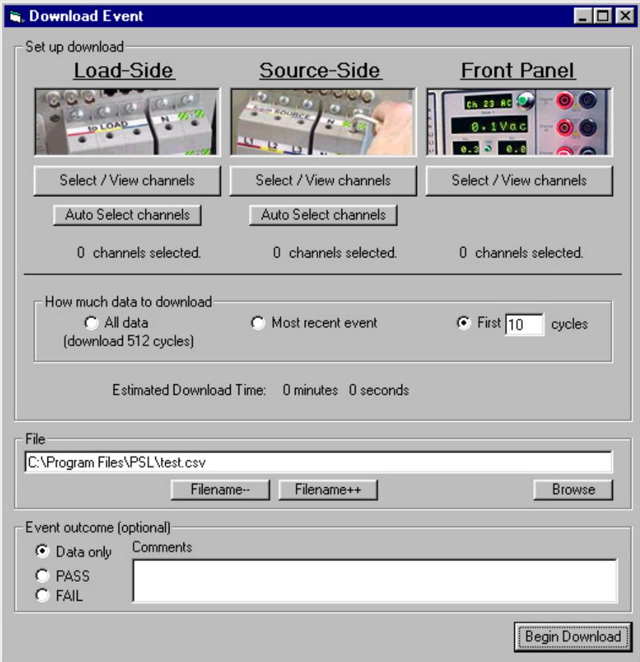
which channels to download, and to re-name the channels. It is helpful to keep the channel names to 5 characters or less, for example "+24V". These new names will appear on your IPC's front panel meters, the on-screen meter, and on the ChannelScope waveforms, making it much easier to keep track of what each channel is used for.
