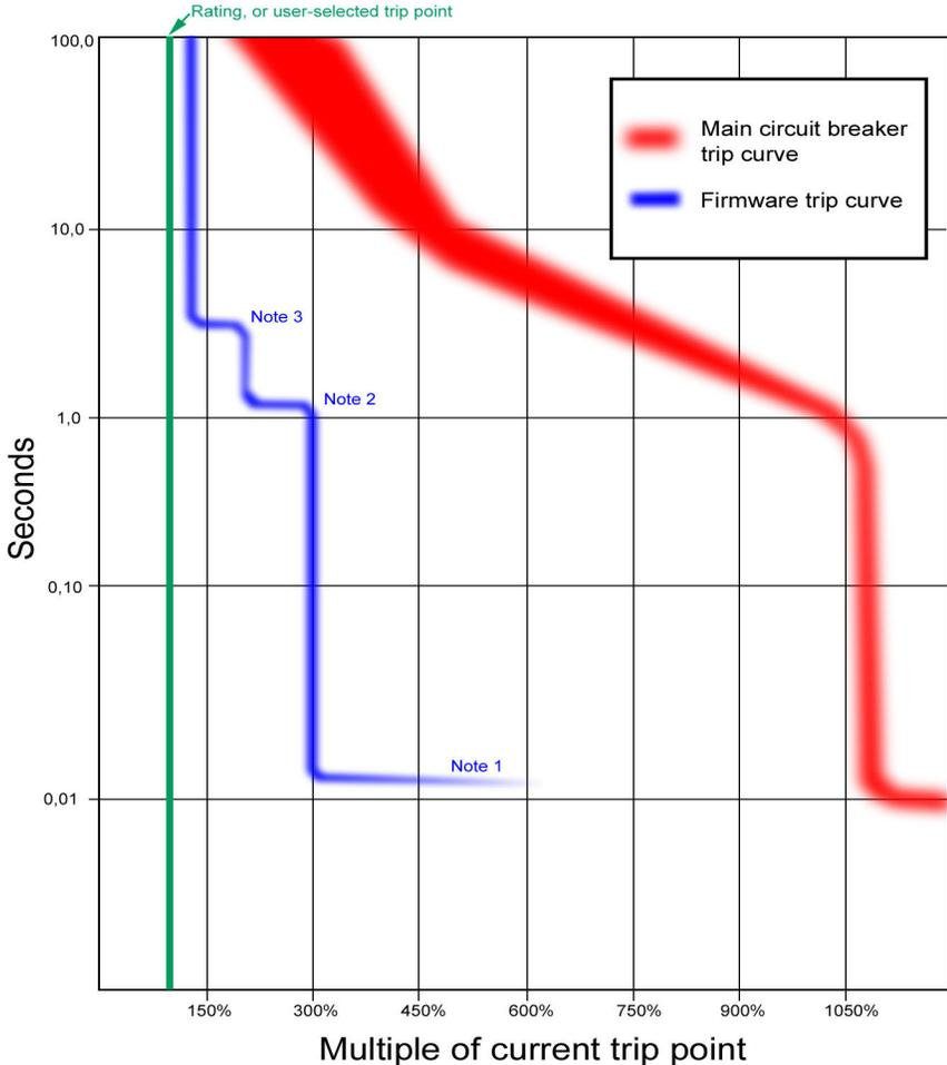
*Note 1: During a sag/swell event, there is a 600-amp instantaneous trip point. On IPC's rated for 200 amps, this trip point can be increased to 700 amps by placing the IPC into Combat Mode.*
