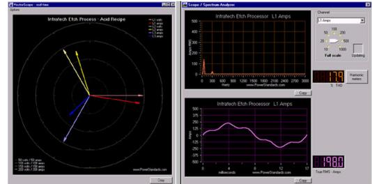
*The Power Flow Analysis option adds vector scopes, spectrum analyzers, harmonics meters, and every imaginable kind of power flow meter - kWh, power factor, kVAR, THD, and much more.*
