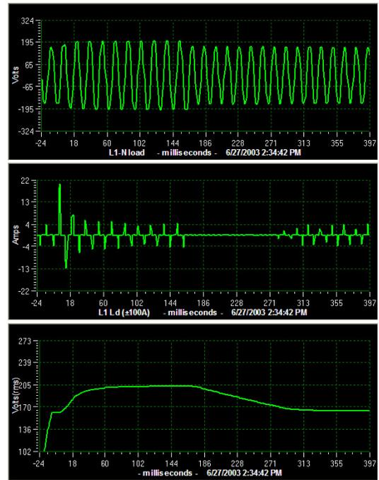
A typical voltage swell, generated by the IPC. The top graph shows the voltage waveform. The middle graph shows the current drawn by the load. The bottom graph shows the response of the load's internal DC bus.
