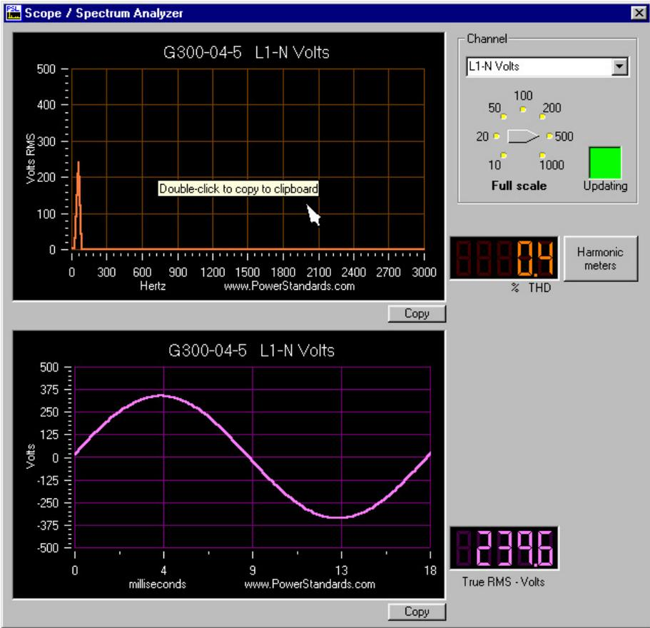
To see individual harmonics, click on the "Harmonics meters" button. The "copy" button places the present value in all of the harmonic meters onto your computer's clipboard, formatted as simple text.
