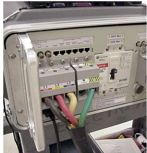
*Typical three-phase source-side connections for a 3-phase delta system. The conductors are large enough to be securely captured by the gray terminal blocks.*
