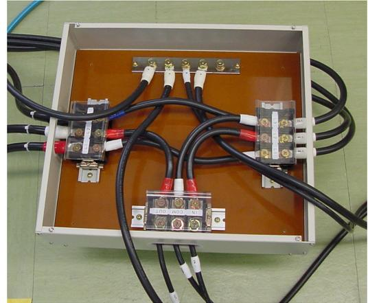
*The wiring for inserting your IPC can be as simple as an extension power cord, broken in the middle, or as sophisticated as a formal junction box such as this one.*
