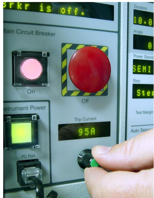
*The IPC main circuit breaker can be manually tripped using the large red mushroom switch. The trip current for this breaker can also be set using the Trip Current dial. For more information, see the Appendix.*
