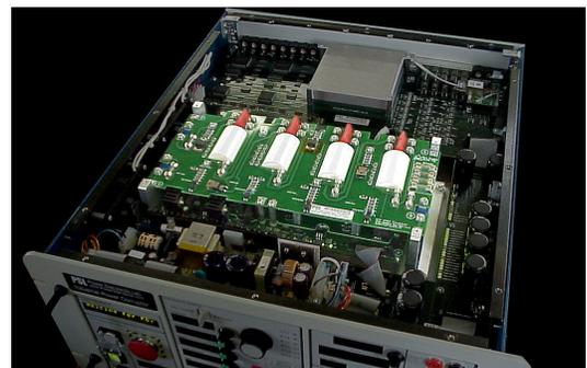
The IGBT module provides gapless switching during transitions.
