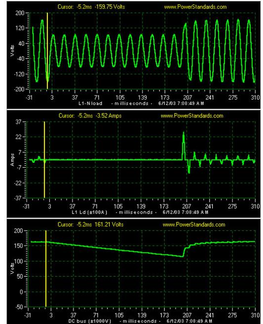
A typical voltage sag, generated by the IPC. The top graph shows the voltage waveform. The middle graph shows the current drawn by the load. The bottom graph shows the load's internal DC bus, which collapsed during the sag. All of these graphs were recorded by the IPC's internal data acquisition system.
