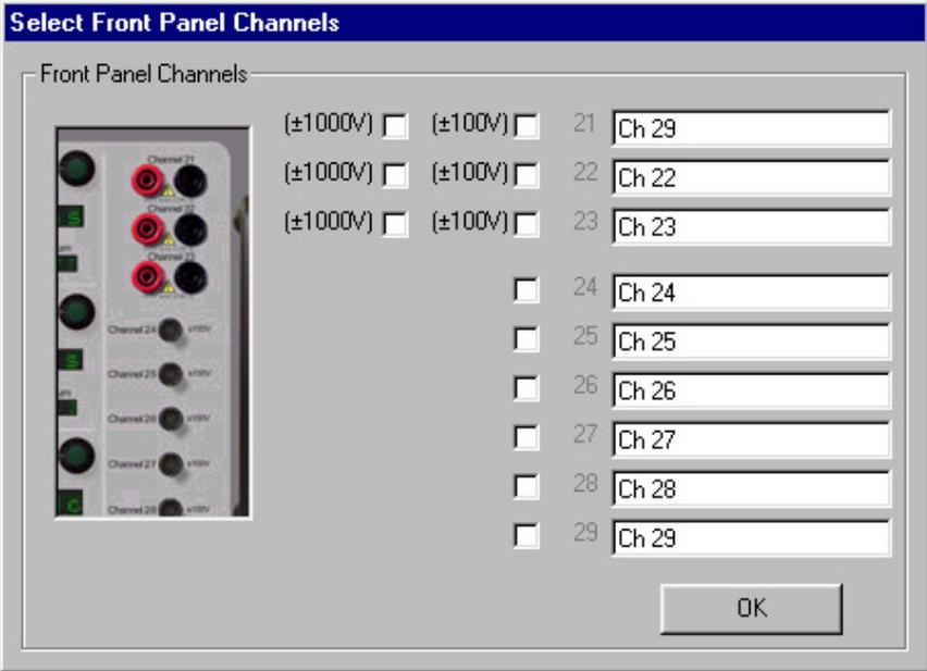
You can re-name the front panel channels - use this screen. It makes sense to limit the names to 5 characters or shorter.
