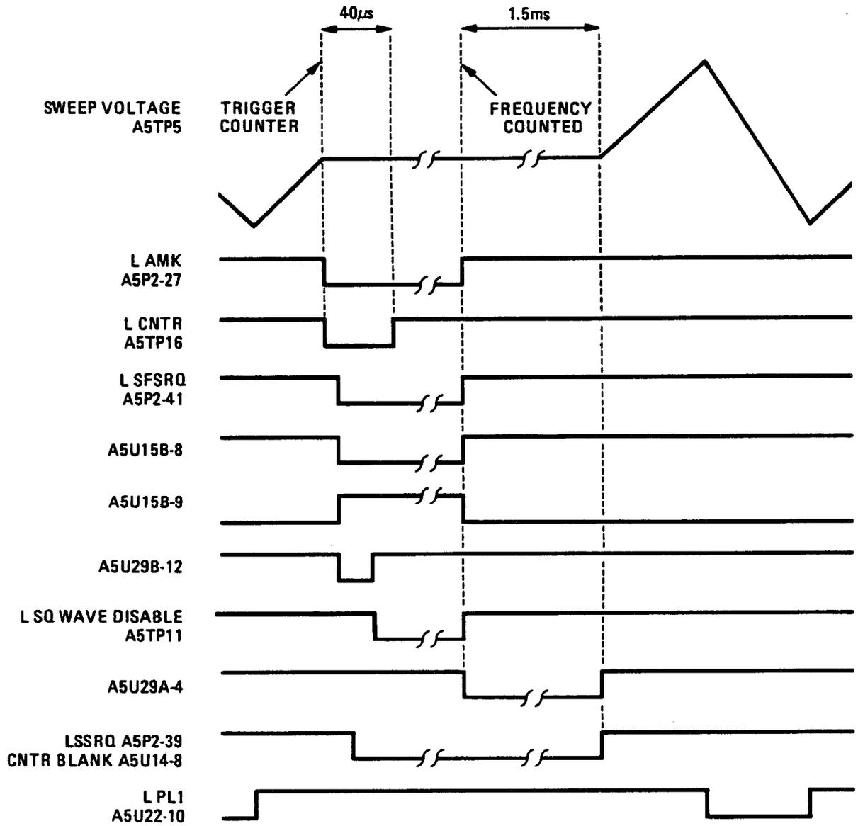
Figure 8-35. Counter Interface Timing Diagram
