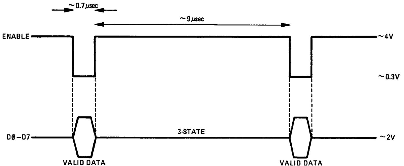
Figure 8-4. Hex Addressed Fast Read — Timing Diagram
