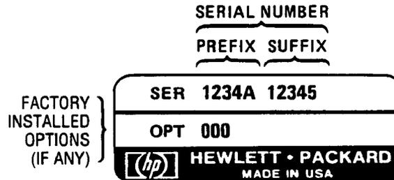
Figure 1-2. Typical Serial Number Plate
