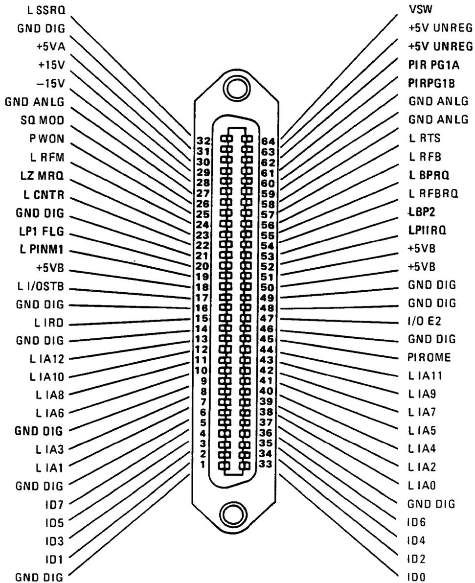
Figure 8-55. Interface Signals on Connector J2
