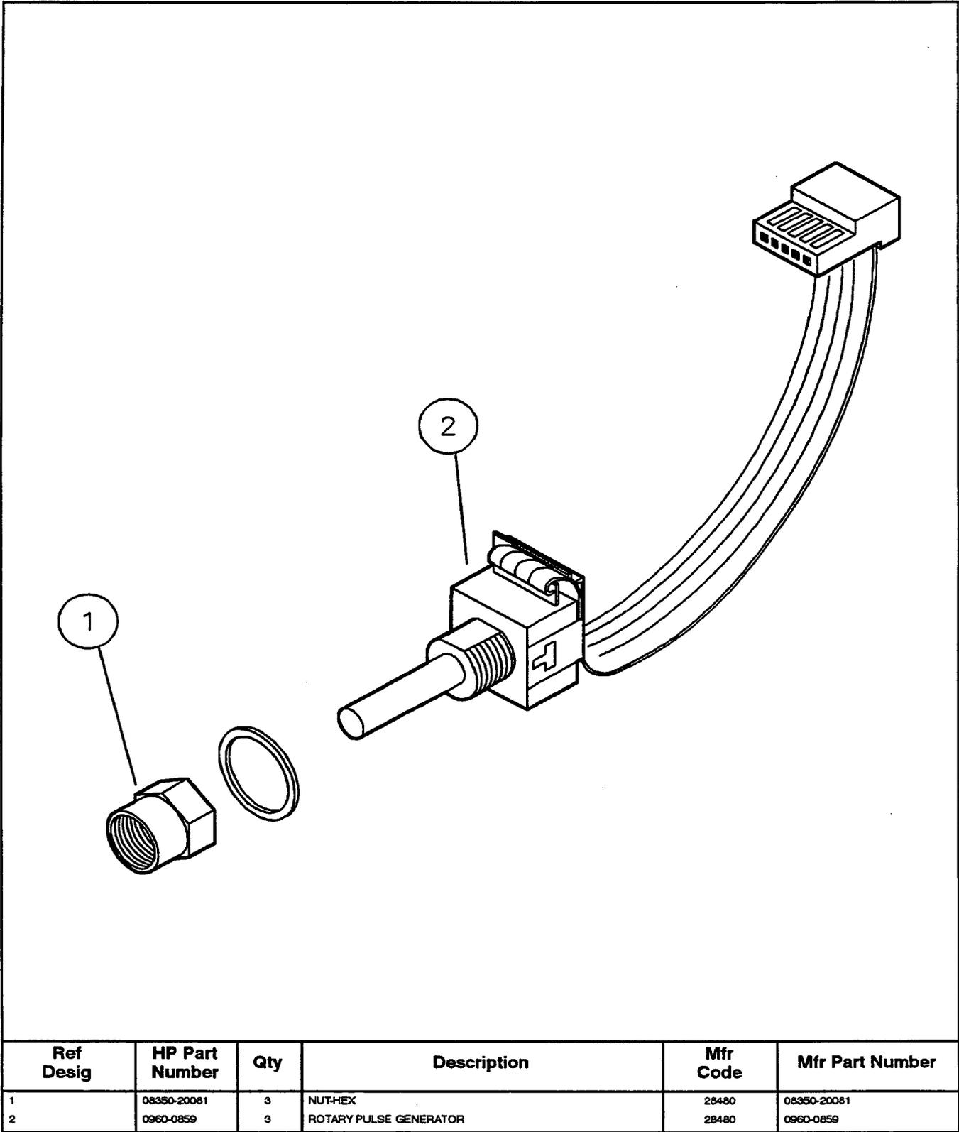
Figure 6-1. Rotary Pulse Generator (RPG), Parts Identification
