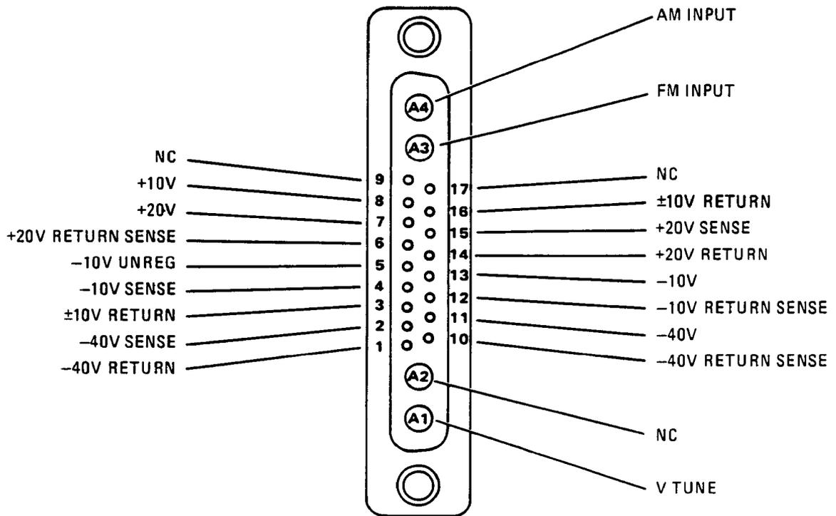
Figure 8-54. Interface Signals on Connector J3
