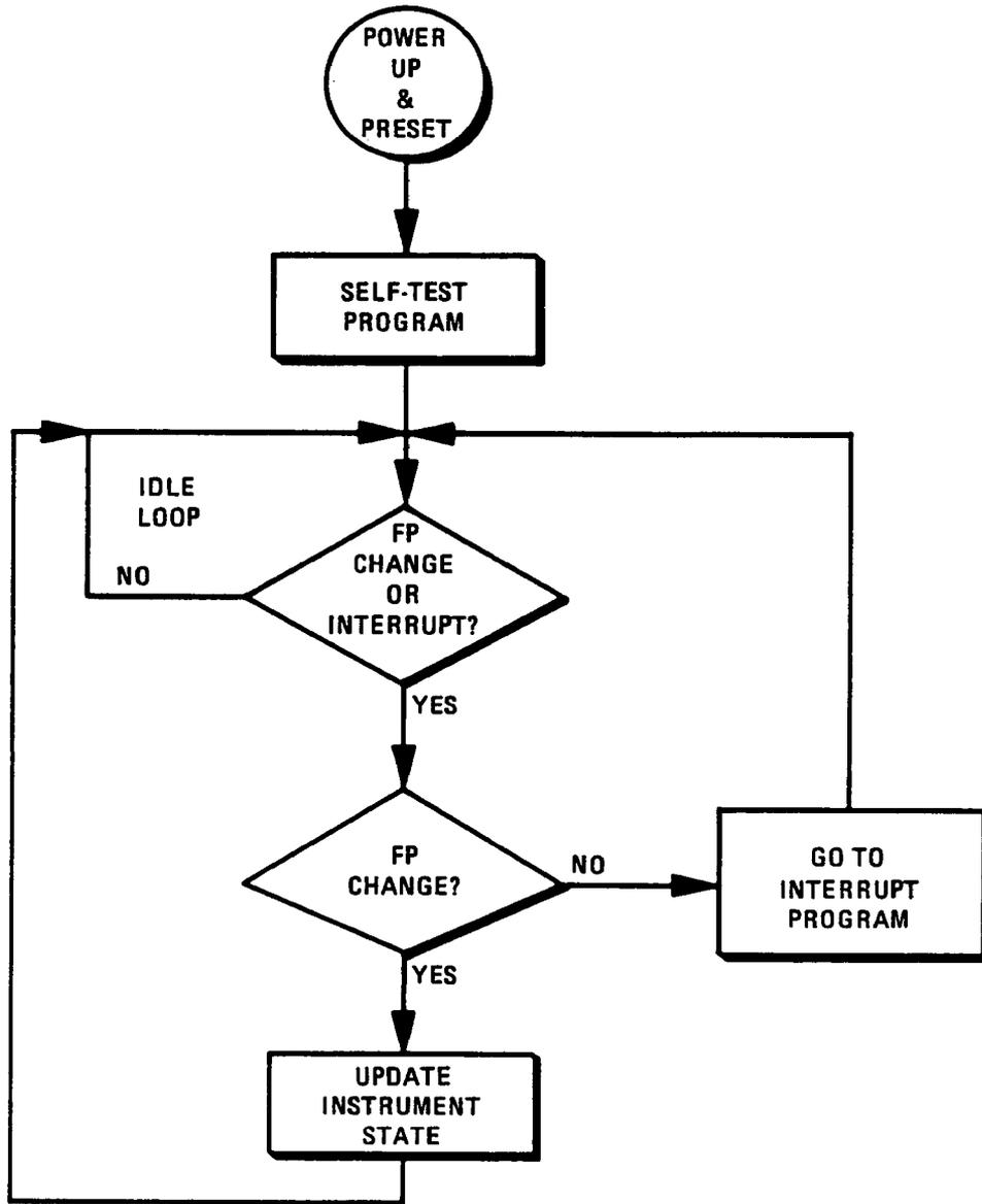
Figure 8-18. HP 8350B Simplified Program Routine (1 of 2)
