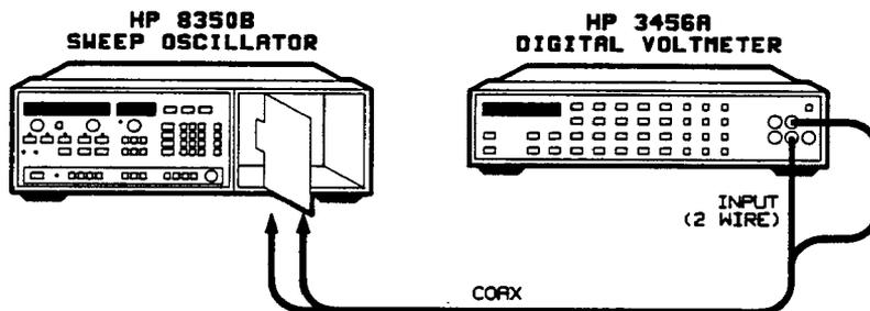
Figure 4-1. Power Supply Test Setup
