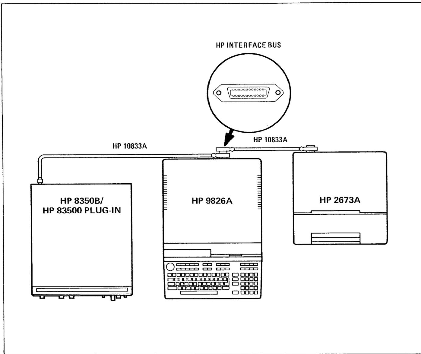
Figure 1. System Connection
