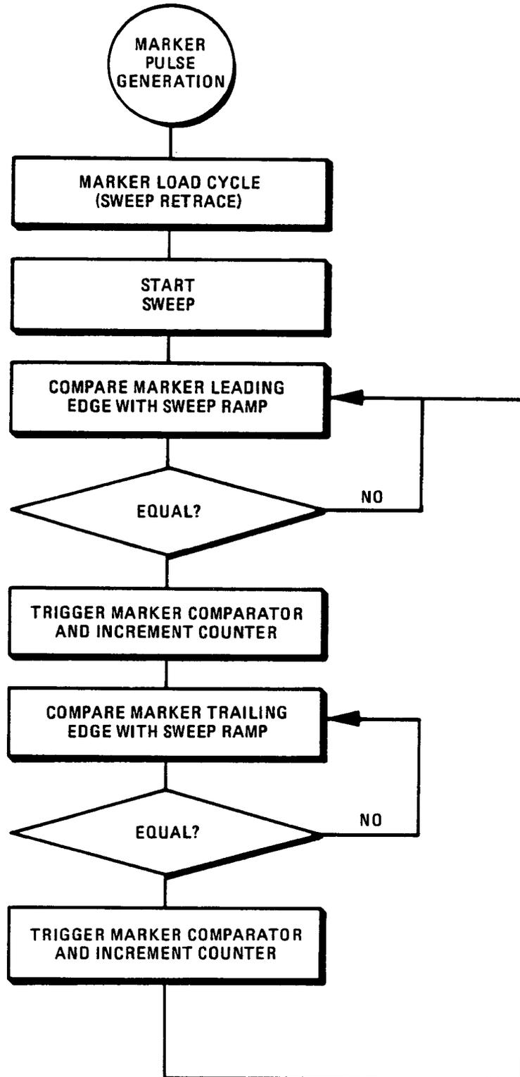
Figure 8-24. Marker Pulse Generation, Flow Diagram
