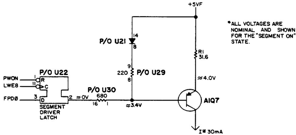
Figure 8-7. Typical Segment Driver Schematic
