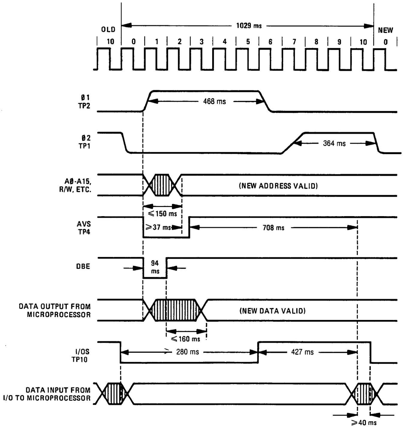
Figure 8-20. A3 Microprocessor Read/Write Timing Diagram
