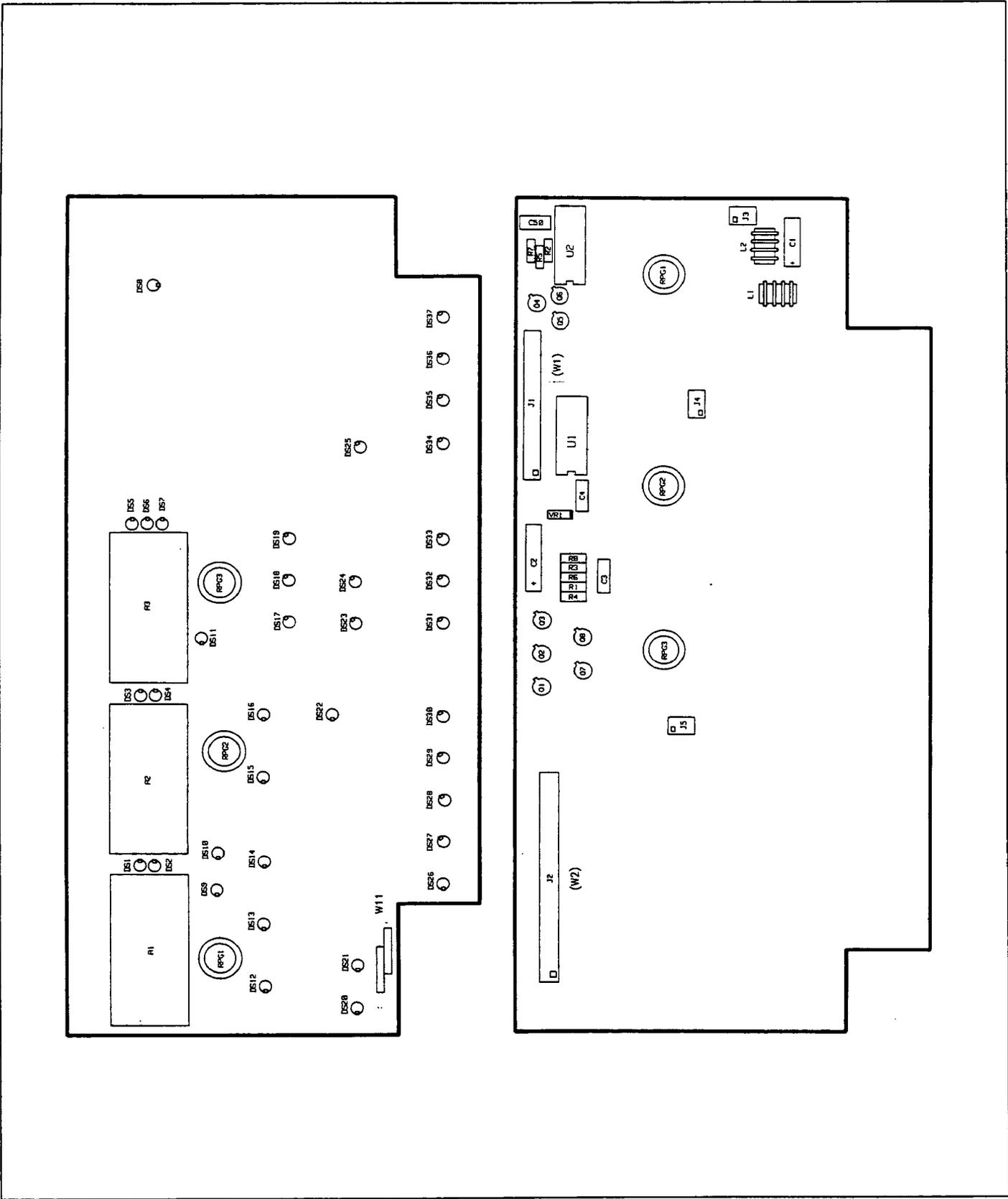
Figure 8-10. A1 Front Panel, Component Locations
