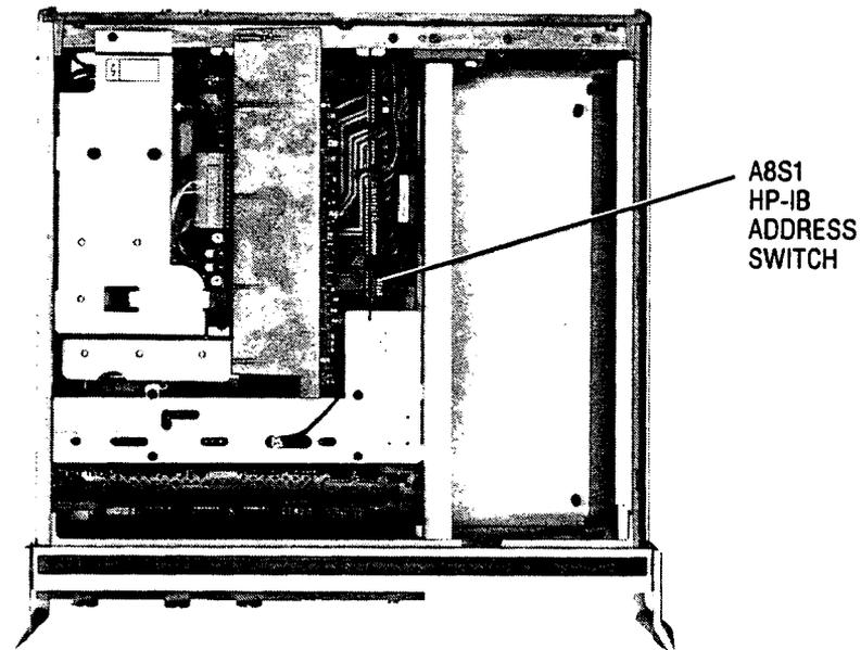
Figure 2-2. Location of A8S1 HP-IB Address Switch
