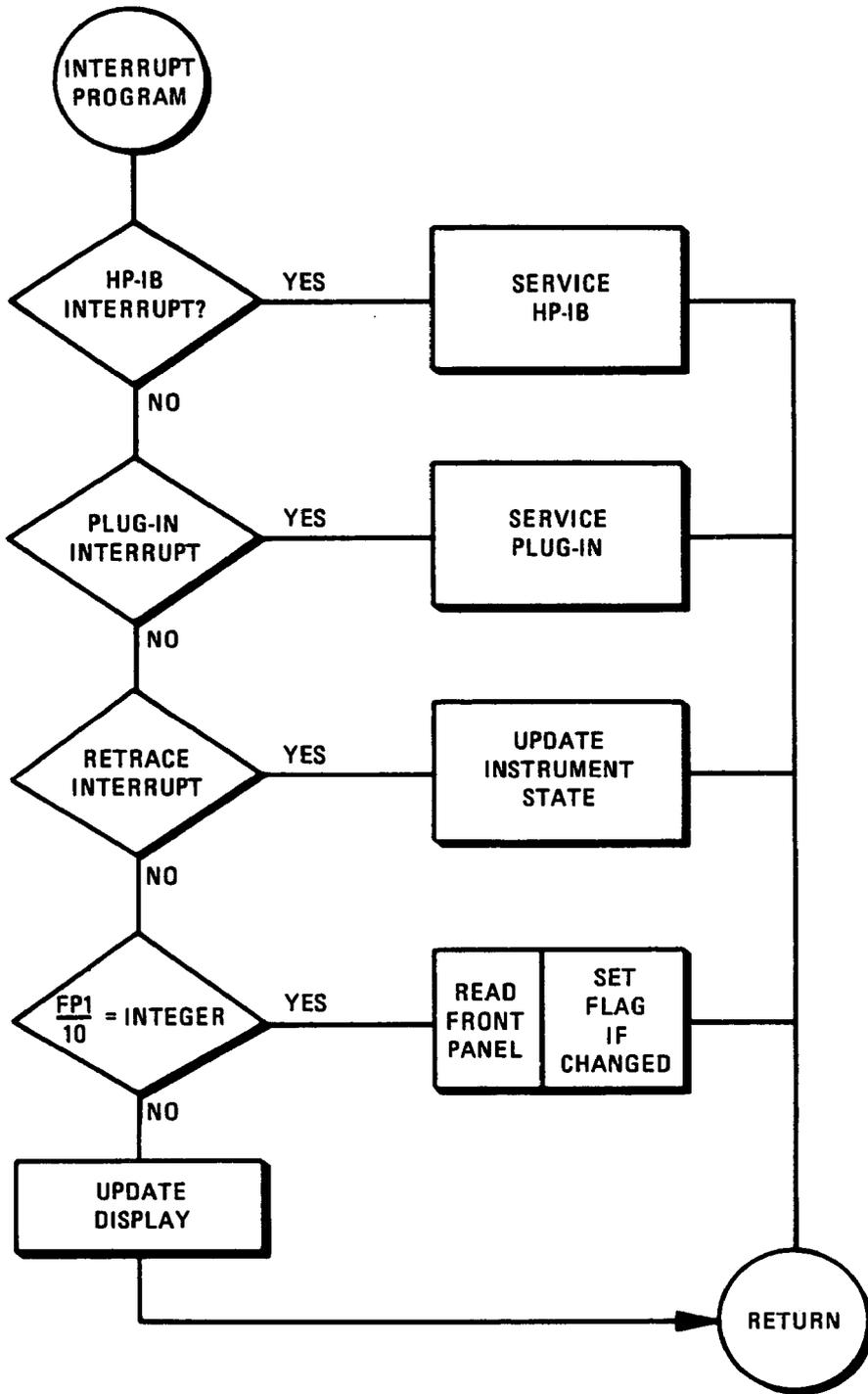
Figure 8-18. HP 8350B Simplified Program Routine (2 of 2)
