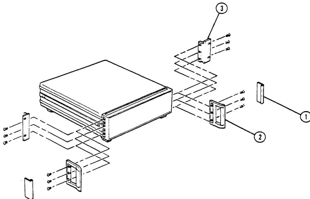
1. REMOVE RACK MOUNT FLANGE (3) AND/OR FRONT HANDLE ASSEMBLY. (1)(2).
