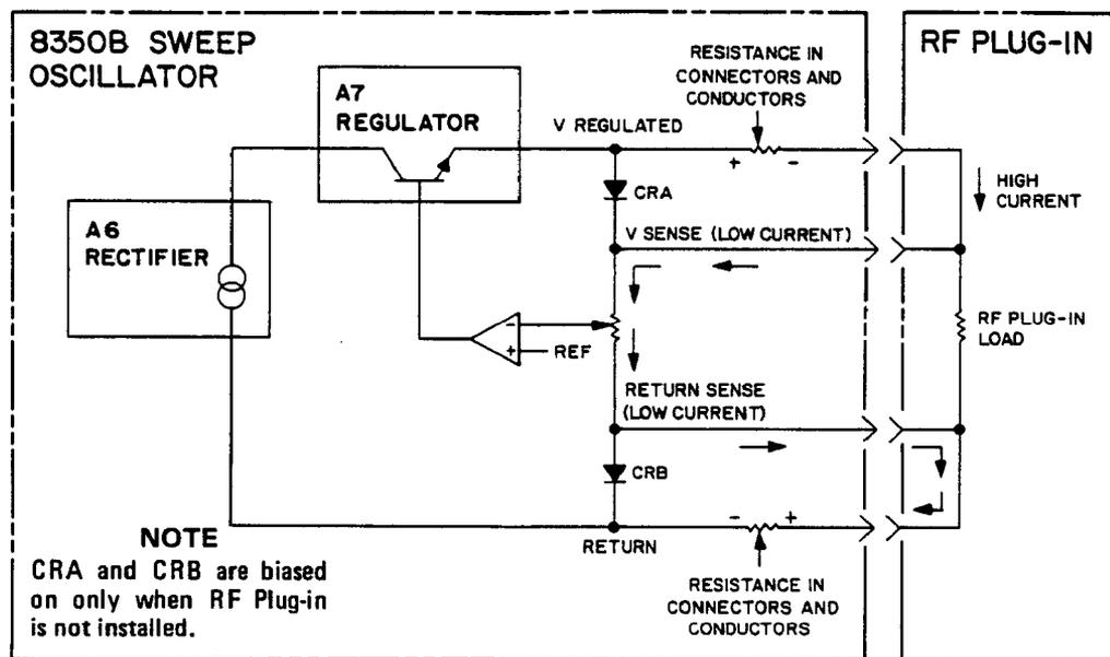
Figure 8-39. Typical Post Regulated Power Supply, Simplified Schematic
