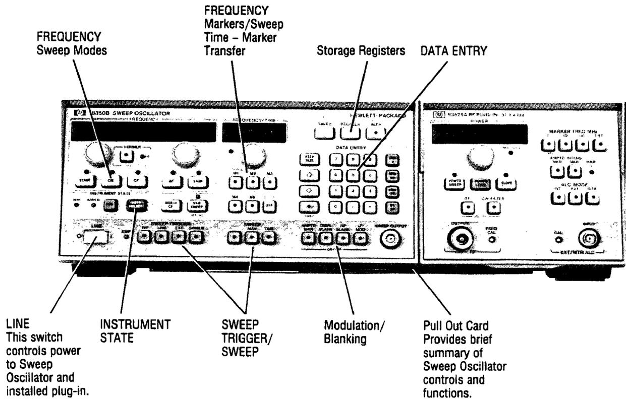
Figure 3-1. Front Panel Features
