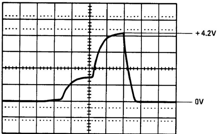
Figure 8-34. Sweep Voltage Waveforms for Sweep versus Marker Self Test
