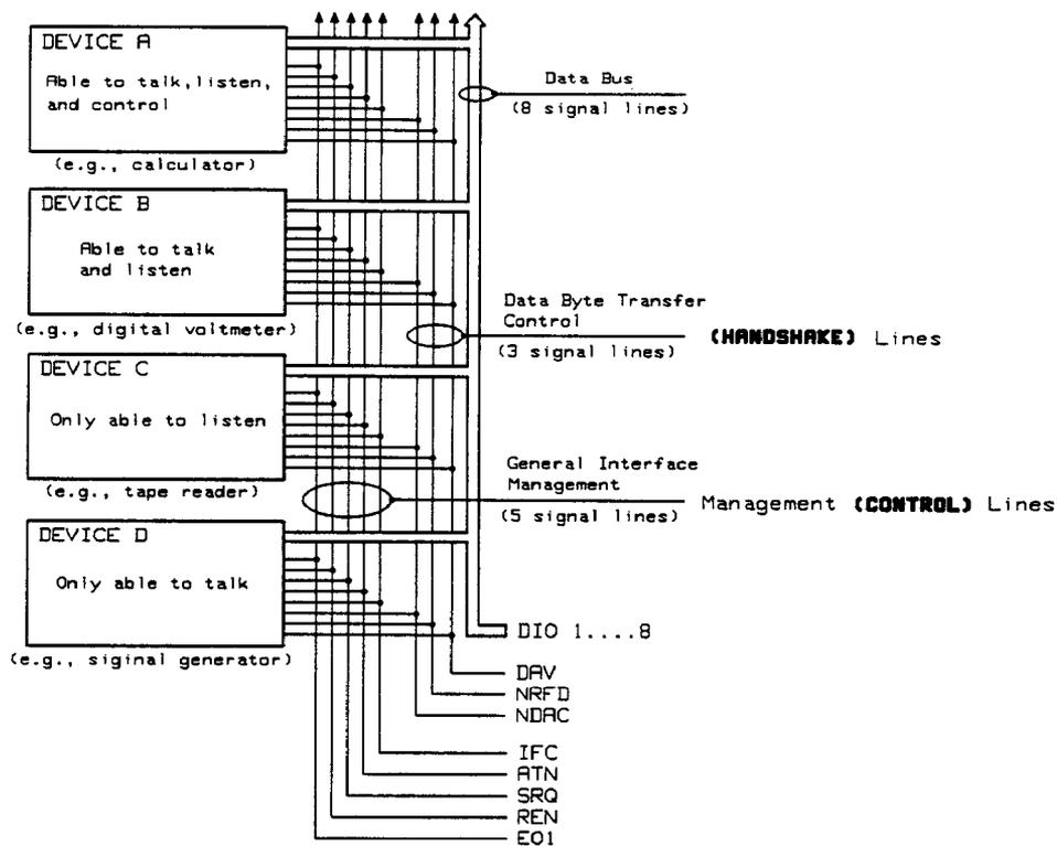
Figure 3-5. Interface Connections and Bus Structure
