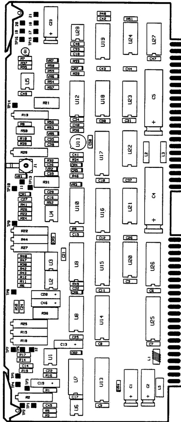
Figure 8-30. A4 Scaling and Marker Component Location Diagram
