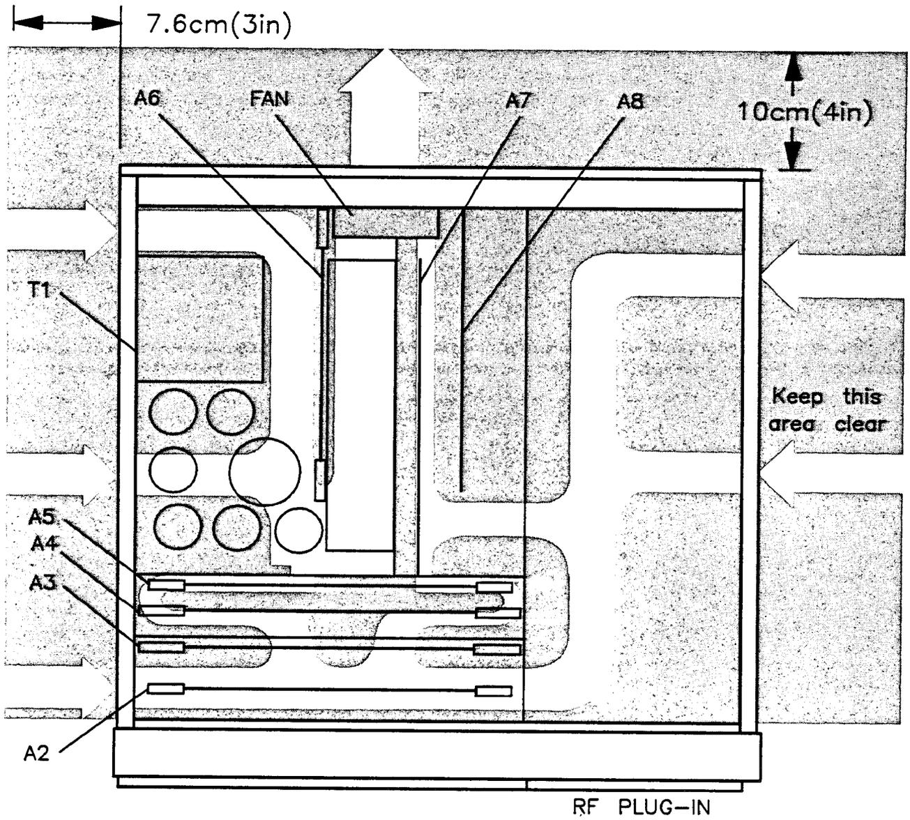
Figure 2-8a. HP 8350B Ventilation Clearances Airflow (Option 400)
