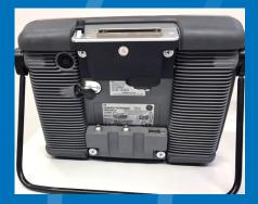
For maximum flexibility, Mentor UT can be configured with an industry standard Tyco or Ipex PA probe connector.
