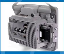
For maximum functionality, attach the MUX module and gain 32:128 capability, an additional hot swappable battery, and standard Tyco connector.
