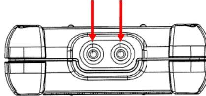
**Note:** Polarity is not a concern for HART connections. Therefore, both jack collars are black.
