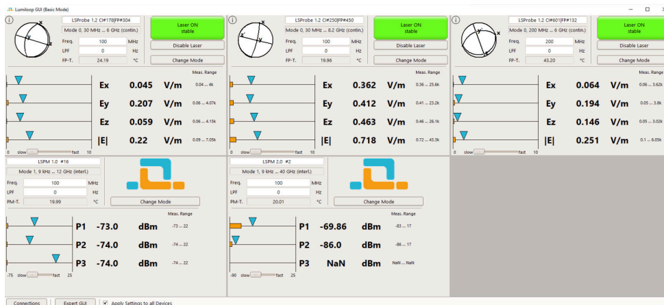
Figure 35: LUMILOOP GUI in Basic Mode resized to fit all connected device frames
