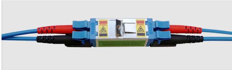
Figure 68: E2000 coupler of sacrificial optical cable assembly
