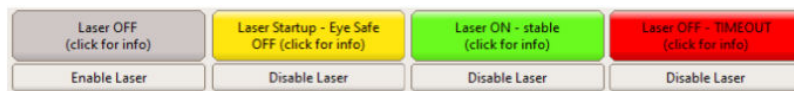
Figure 37: LUMILOOP GUI laser indicator when off, during start-up, in safe operation and upon encountering a time-out error
