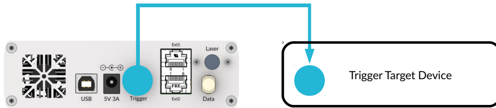
Figure 15: External trigger output using BNC connector
