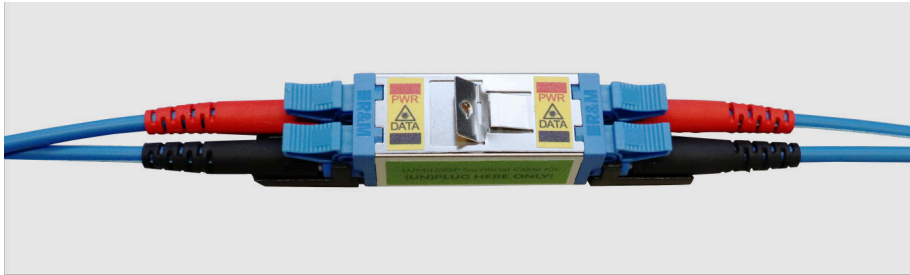
Figure 26: E2000 coupler of sacrificial optical cable assembly
