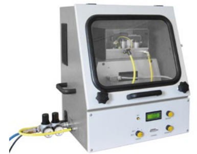
Model 3413U: Dust aerosol generator inside full enclosure for difficult powders
