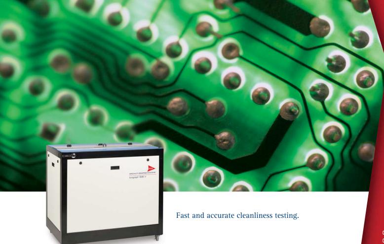
Specialty Coating Systems' name is synonymous in the industry with automated ROSE (Resistivity of Solvent Extract) testing systems. SCS Ionograph® ionic contamination test systems utilize the dynamic extraction method to measure resistivity change when a substrate is submerged in the ultra-pure test solution. The degree of change in resistivity indicates the level of contamination, which is often the result of residues from fabrication and board assembly processes.
