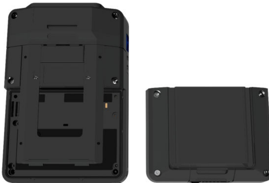
Figure 2-9: Trex unit with the power module removed
