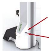
USB, RS2232 and TTL outputs to connect the stand to a computer or an automaton
