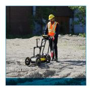
Detect metallic and non-metallic pipes and cable
