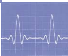
Sequence mode (in C.C mode and fast-speed mode) H: 5 ms/div, V: 10 A/div
