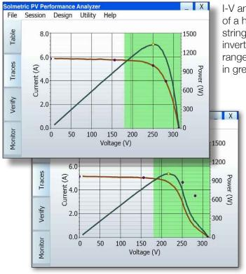
I-V and P-V curves of a healthy PV string. Start/Stop inverter voltage range is highlighted in green.
