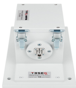
PCJ 9202 calibration jig, side view
