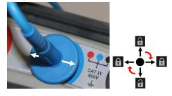
With the arrows on the plug finger guard horizontal on the instrument as shown to lock. Twist 90° to to unlock. In addition, for the same reason, the test clips are not removable from the test lead.
