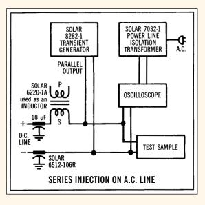
**Power Current in Series Injection Mode:** Handles up to 50 amperes of current at power frequencies.
