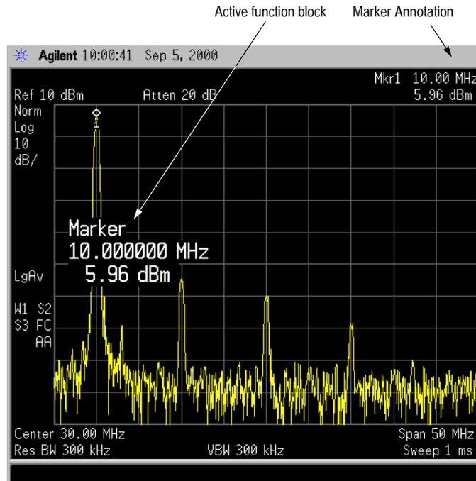
**Figure 3-4 Relationship Between Frequency and Amplitude**
