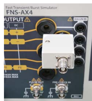
02-00152A adapter mounted onto L2(N.-) port of EUT LINE OUTPUT
