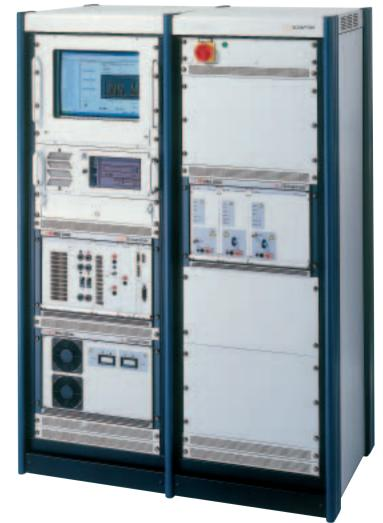
**NSG 5200.** Designed to be used either alone or in combination with an NSG 5000 system, the NSG 5200 is designed to simulate events that include voltage dropouts, sine waves and other events superimposed on the automotive battery: Dips and Drops, Starting Profiles, and Sinusoidal Noise. Additionally, the NSG 5200 may be configured for magnetic field immunity testing. A basic configuration of the NSG 5200 would be with one
