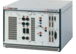
**Basic Chassis NSG 5201 and NSG 5202.** The 19" basic chassis contains all the power supply components and, if required, the burst-transformer, the rear-facing fans, the control and signal bus boards as well as the common inputs and outputs for the safety circuits and signals for the expanded control and monitoring of the test procedures.
