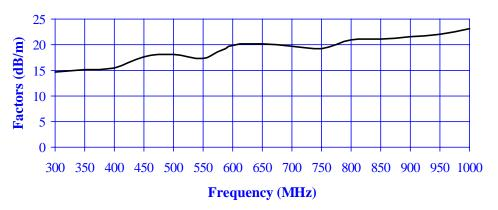
Field strength (dB/m) = Output measured (dBV) + Antenna Factor (dB/m)
