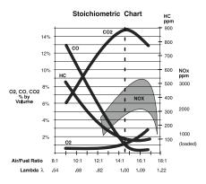
In reality, the air we breath and the fuel used are not pure, and the spark may not occur at precisely the right moment. Subsequently, the exhaust stream will contain hydrocarbons (HC), and carbon monoxide (CO), in addition to Carbon Dioxide (CO2) and traces of Oxygen (O2), Oxides of Nitrogen (NOx), Sulfur Dioxides (SO2) and soot.
