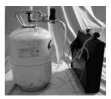
The analyzer will zero the gas bench then ask you to turn on the gas valve on and adjust the pressure regulator until the bar graph is between the two arrows.
