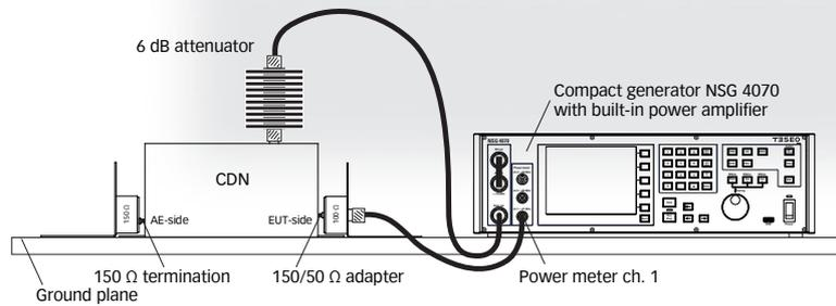
Application for IEC/EN 61000-4-6, EUT set-up with CDN
