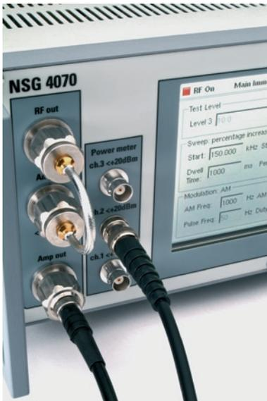
NSG 4070 front panel with RF ports
