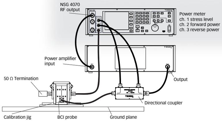
Application for automotive BCI, EUT set-up with monitoring probe
