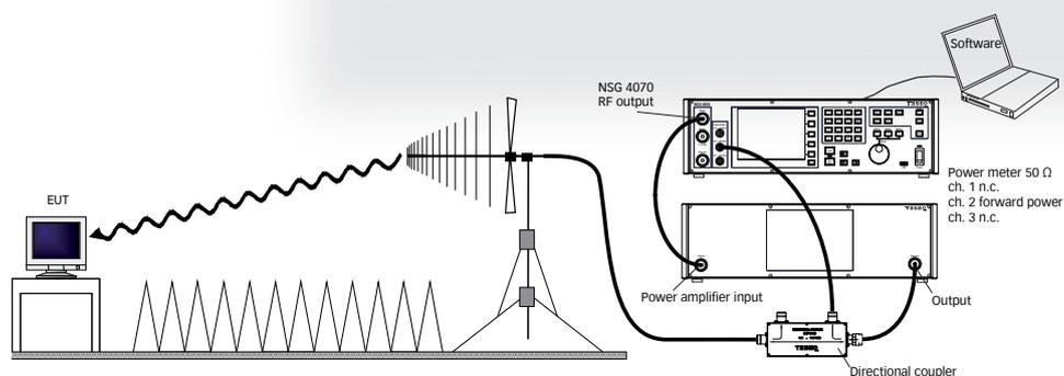
Application for IEC/EN 61000-4-20 up to 1 GHz (power requirements and frequency range demand external power amplifier and directional coupler, field probe control required optional software)
