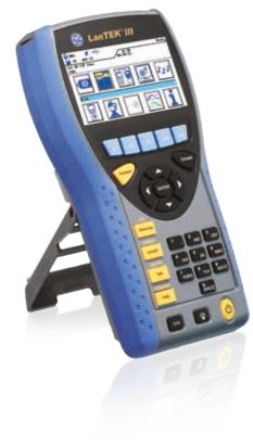
The LanTEK III is an easy to use cable certifier that meets existing TIA and ISO/IEC performance requirements for testing up to Cat 7A/1000MHz. FiberTEK III adapters are used with LanTEK III for fast and simple certification of high bandwidth single-mode and multimode fiber optic cabling including support for encircled flux testing.
