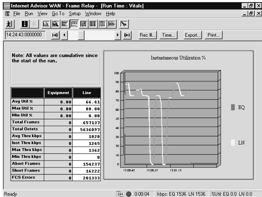
Figure 2. Vitals provides real-time measures of network conditions.
