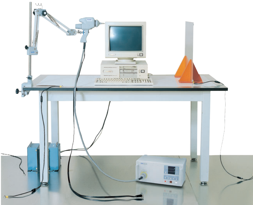
Test set-up example with ESS-801
