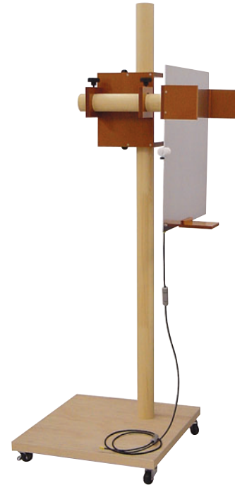
ESS-801GL (Vertical coupling plane & Cable with resistors)
