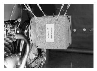
• Clearance hole through armature and shaker allows unlimited positioning along the axis of the stinger
