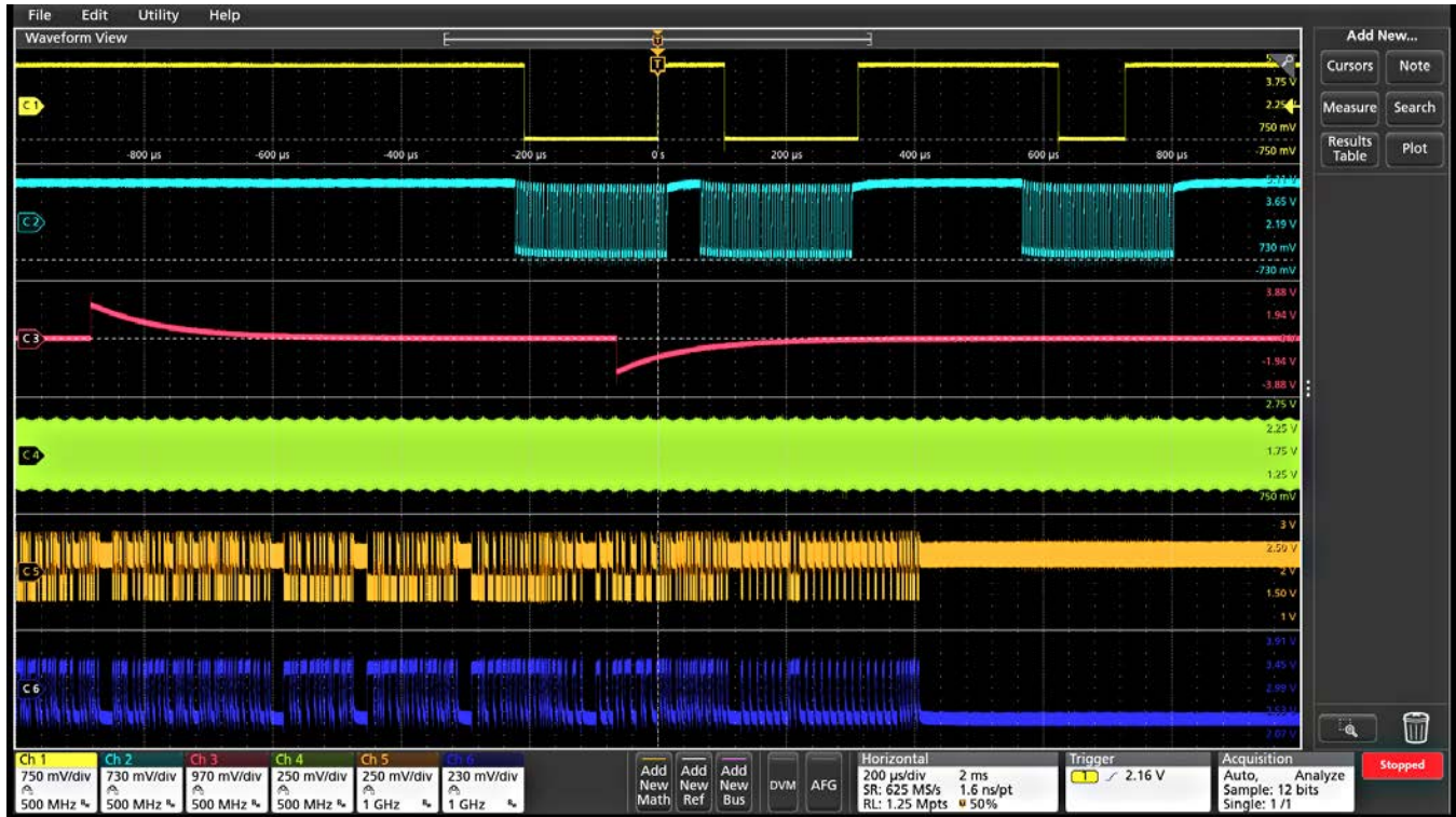
Figure 6: Stacked display mode enables easy visibility of all waveforms while maintaining maximum ADC resolution on each input for the most accurate measurements.
