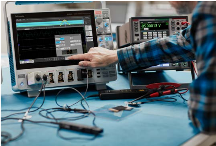
Figure 9: Interact with the capacitive touch display in the same way you do on your phones and tablets.
