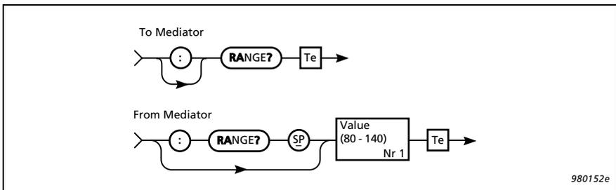
Fig. 11.29 Syntax for the **R**ANge? query message and Mediator response
