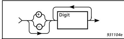
*Fig. 11.4 Syntax for numerical data of type NR1*
