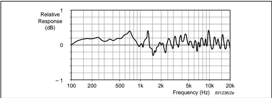
*Fig.9.5 Effect of Mediator's casing on frequency response*
