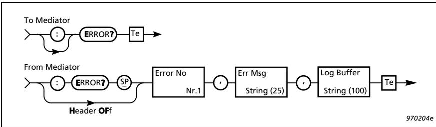
*Fig. 11.13 Syntax for Error? query and amplifier response*
