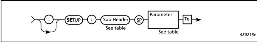
*Fig. 11.32 Syntax for the **SE** setup command*
