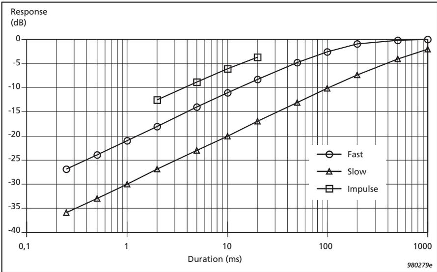
Fig.9.4 Curves showing the detector response of Mediator to 4kHz tone bursts of various durations
