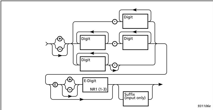
*Fig. 11.5 Syntax for numerical data of type NR3*
