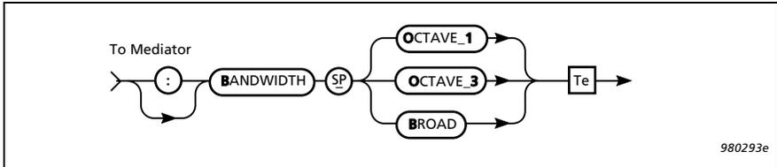
Fig. 11.10 Syntax for **B**andwidth command
