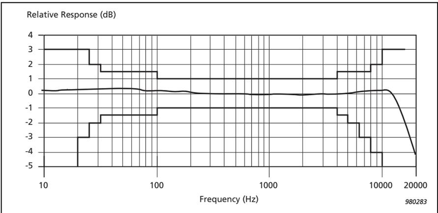
*Fig.9.6 Free-field frequency response of Mediator fitted with the supplied microphone Type 4188. IEC 651 Type 1 tolerances are also shown*
