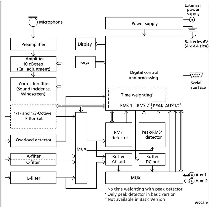
*Fig. 1.1 Simplified block diagram for 2238 Mediator*
