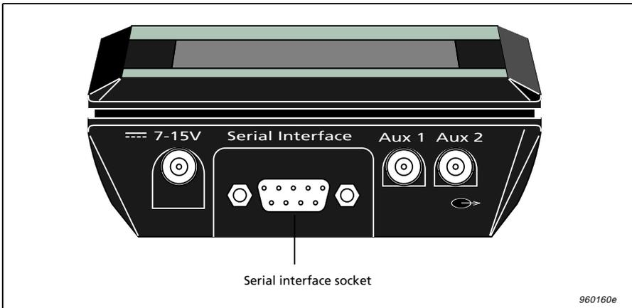
*Fig. 7.1 Location of the serial interface connector*
