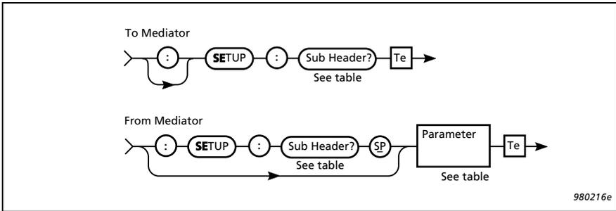
Fig. 11.33 Syntax for the **SETUP?** query and Mediator response
