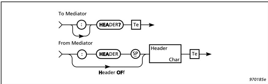
*Fig. 11.9 Syntax for **Header?** query and Mediator response*
