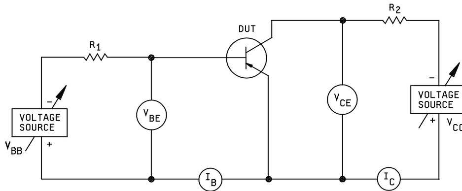
NOTE: For other configurations, the circuit may be modified in such a manner that it is capable of demonstrating device conformance to the minimum requirements of the applicable specification sheet.
