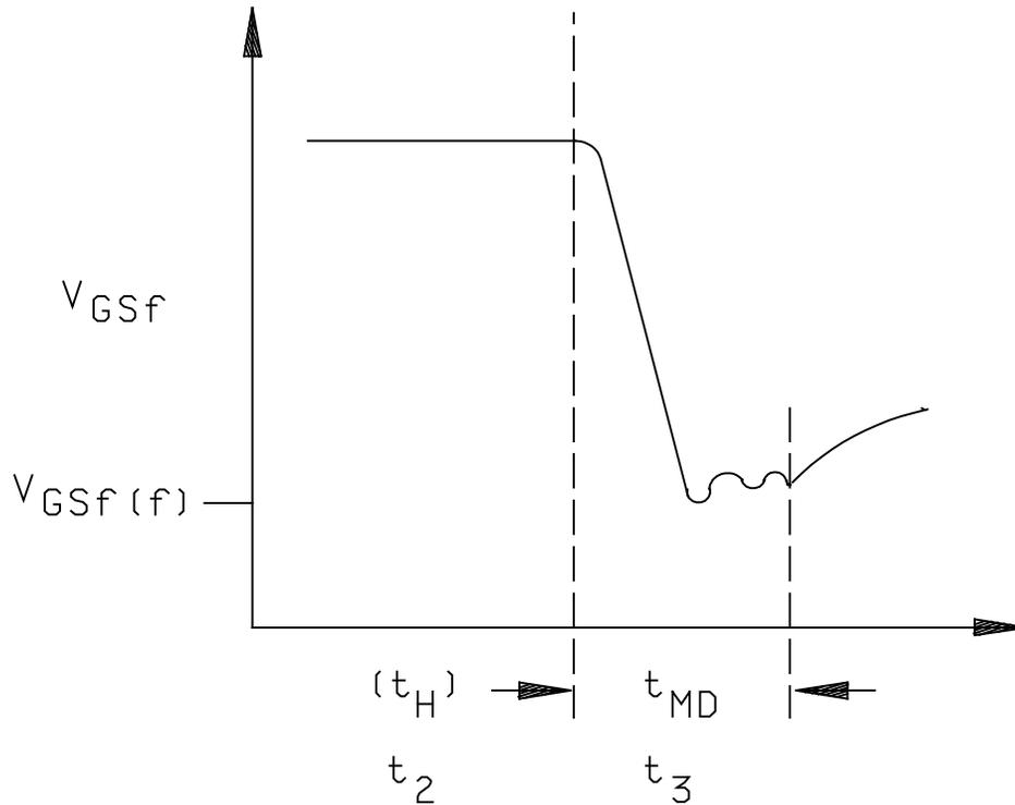
FIGURE 3104-4. Second  $V_{GSf}$  measurement waveform.
