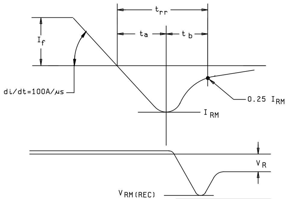
FIGURE 3473-2. Generalized reverse recovery waveforms.
