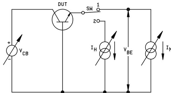
FIGURE 3131-1. Thermal impedance testing setup for transistors.
