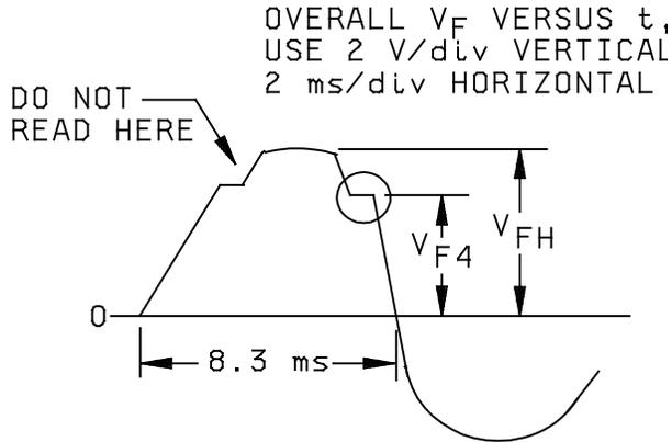
NOTE:  $V_{F4}$  step trace is provided when anti-parallel diodes in circuit briefly commutate off (the ac current passes through zero during each cooling cycle of individual bridge legs under ac test conditions.)
