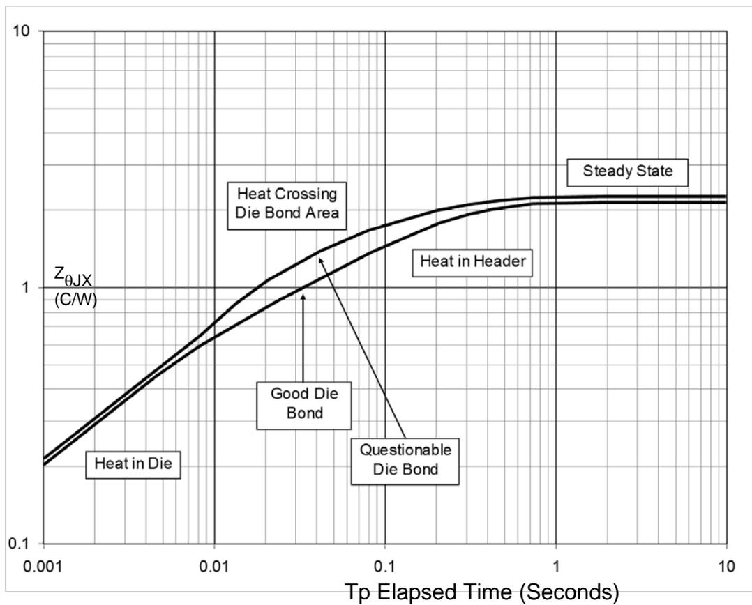
FIGURE 3131-4. Heating curves for two extreme devices.
