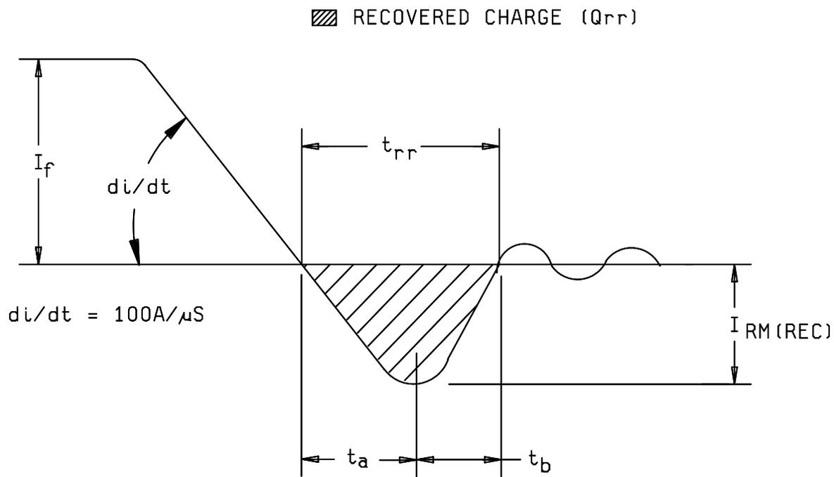
FIGURE 3473-5. Typical  $t_{rr}$  waveform (for mnemonic reference only).
