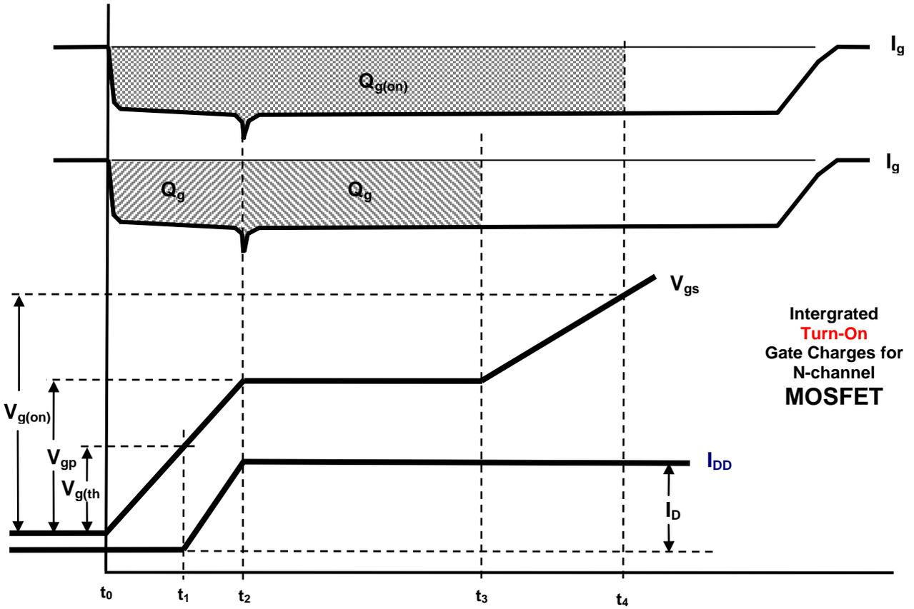
FIGURE 3471-6. Integrated Gate Charges, Condition B (Turn-On).
