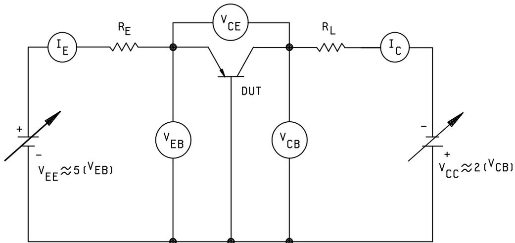
FIGURE 3051-1. Test circuit for SOA (continuous dc).
