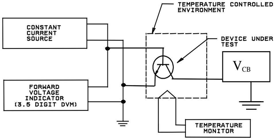
Step 1: Measure  $V_{BE1}$  at  $T_{J1}$  using  $I_M$
