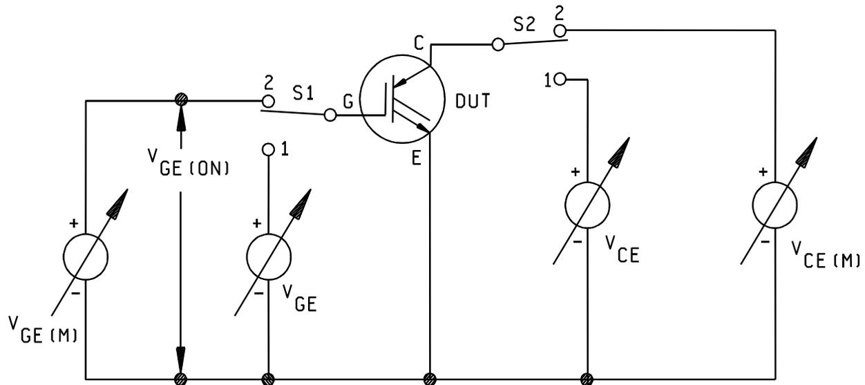
NOTE: The circuit consists of the DUT, four voltage sources, and two electronic switches. During the heating phase of the measurement, switches S1 and S2 are in position 1. The values of  $V_{CE}$  and  $V_{GE}$  are adjusted to achieve the desired values of  $I_C$  and  $V_{CE}$  for the  $P_H$  heating condition.
