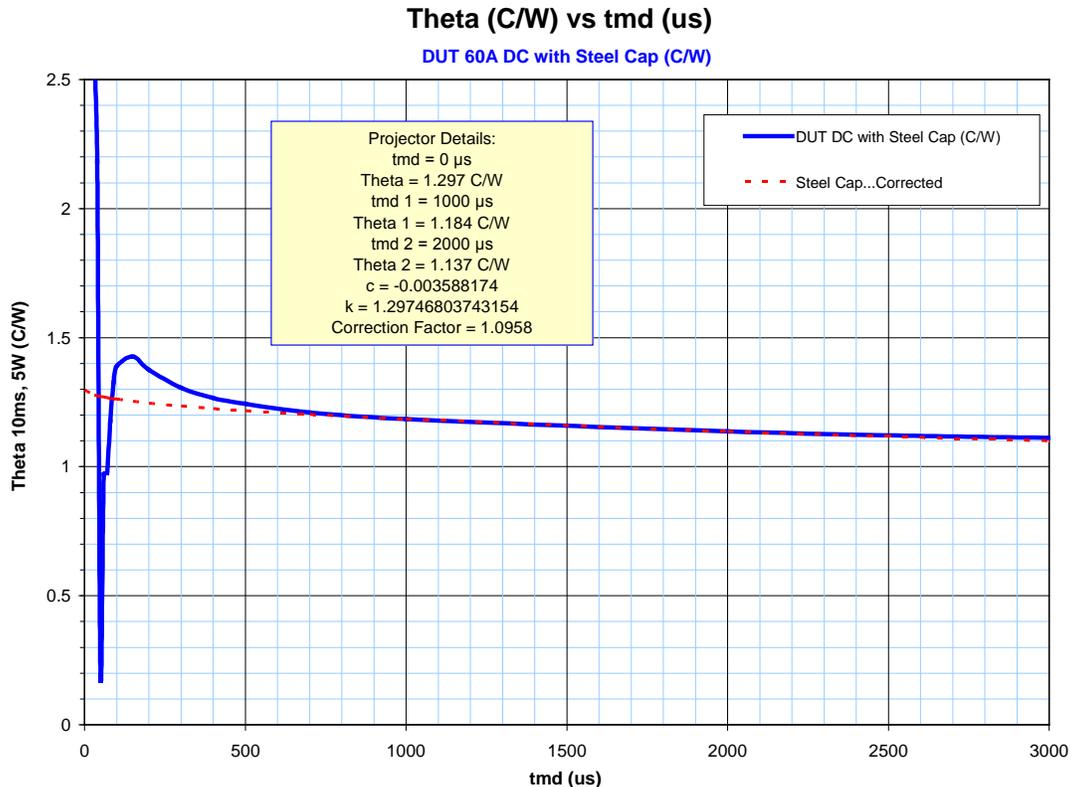
NOTE: Observe closely on the curve above that if you had not used the “projector” calculations and had incorrectly used,  $t_{MD} = 50 \mu s$  (thinking that was close to zero and should be accurate), a measured theta value less than 25 percent of the real theta value. The next measurement would have likely jumped around a little and SPC charts would be plotting setup errors and not product integrity.
