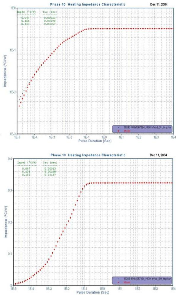
FIGURE 3161-7. Heating curve and thermal model example.
