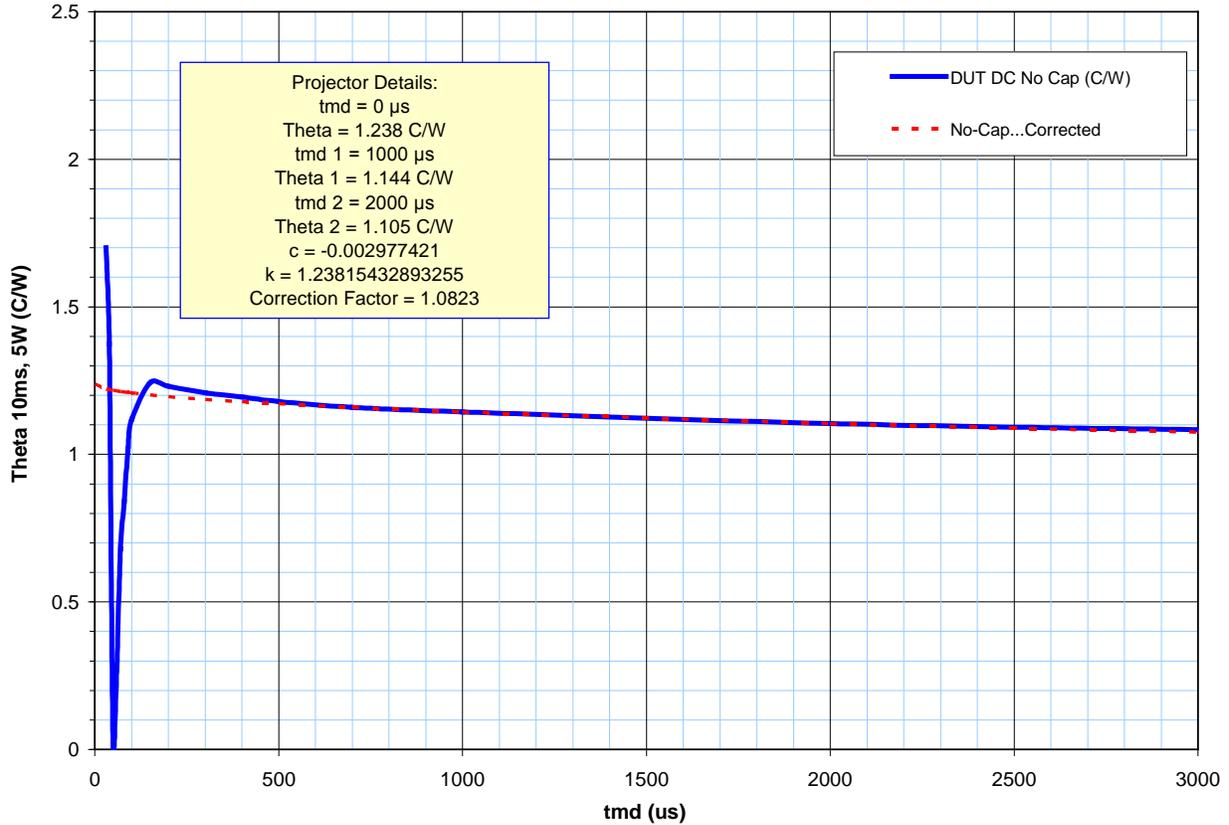
NOTE: The magnetic disturbances removed, there only remains the effects of stored charge and/or recovery delay in the thermal resistance tester as, in this case, the power source must switch from  $I_H = 60\text{ A}$  to  $I_M = 50\text{ mA}$ .
