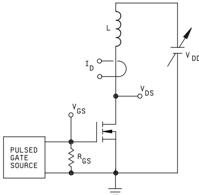
NOTE: The test circuit, shown for n-channel devices, is also applicable for p-channel devices with appropriate changes in polarities and symbols.
