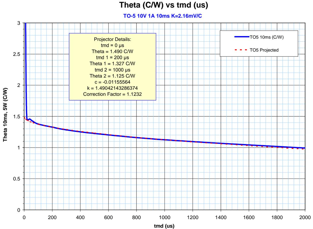
NOTE: Knowing exactly how to select  $t_{MD1}$  and  $t_{MD2}$  is important. Note that  $t_{MD1}$  needs to be selected just past the point where various perturbations occur and can only be accomplished by making “cooling plots” like the ones used for above figure. For  $t_{MD2}$ , choose a value between two and three times  $t_{MD1}$ .
