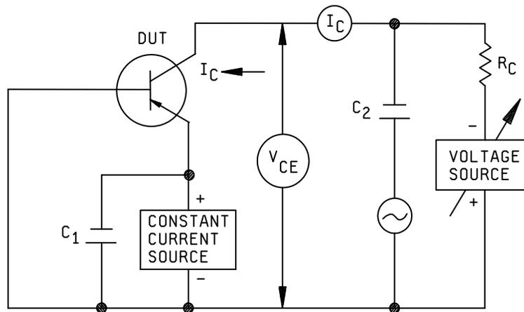
FIGURE 3231-1. Test circuit for small-signal short-circuit output admittance.
