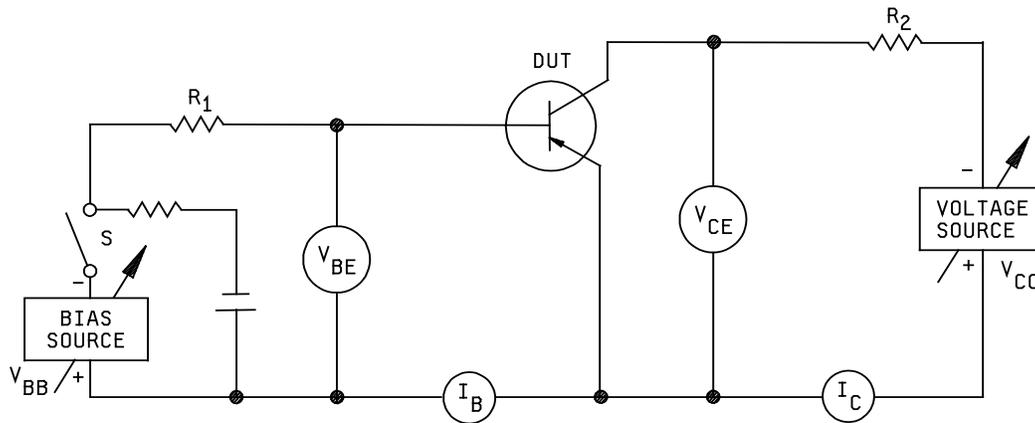
NOTE: If necessary, switch S shall be used to provide pulses of short duty cycle to minimize the rise in junction temperature. When pulsing techniques are used, oscillograph methods shall be used to measure  $V_{BE}$  and other necessary parameters and the duty cycle and pulse width shall be specified.
