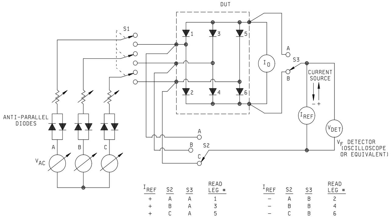
NOTE 1: All voltage measurements shall be made using leads Kelvin-connected directly to the bridge terminals.
