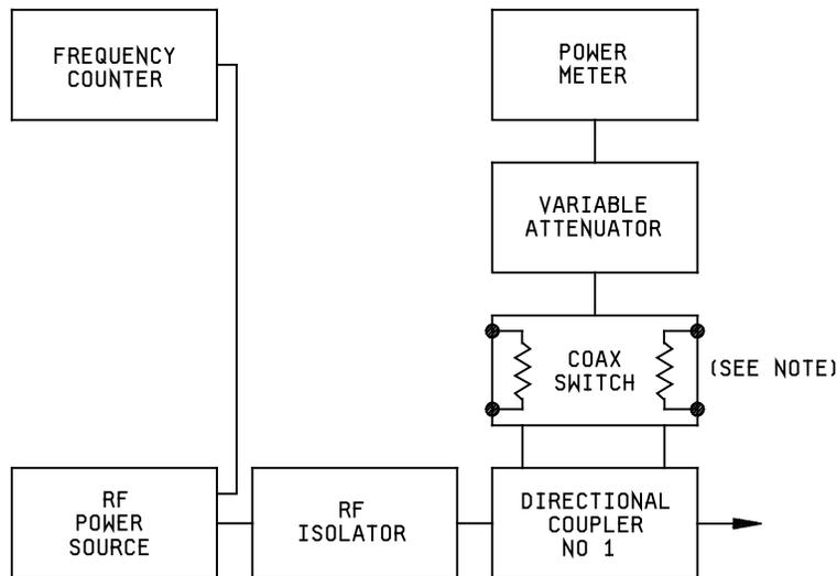
NOTE: The unswitched port automatically terminates the alternate coupler port in  $50\ \Omega$  when using the coax switch specified in the equipment list.
