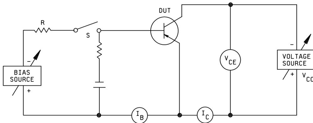
NOTE: The ammeter shall present essentially a short circuit to the terminals between which the current is being measured or the voltmeter shall be corrected for the drop across the ammeter.
