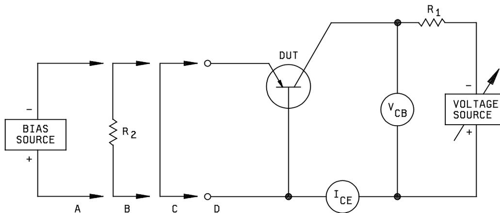
NOTE: The ammeter shall present essentially a short circuit to the terminals between which the current is being measured or the voltmeter shall be corrected for the drop across the ammeter.
