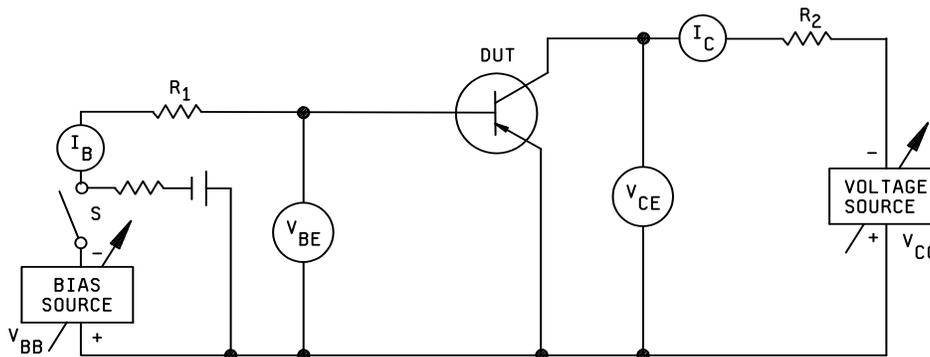
NOTE: If necessary, switch S shall be used to provide pulses of short duty cycle to minimize the rise in junction temperature. When pulsing techniques are used, oscillograph methods shall be used to measure  $V_{BE}$  and the other necessary parameters and the duty cycle and pulse width shall be specified.
