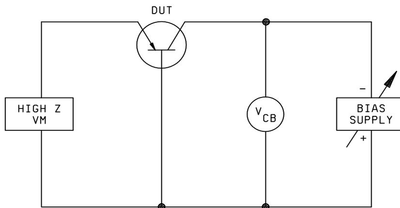
NOTE: The circuit shown is for measuring the emitter floating potential. For other device configurations, the above circuitry should be modified in such a manner that is capable of demonstrating device conformance to the minimum requirements of the individual specification sheet.
