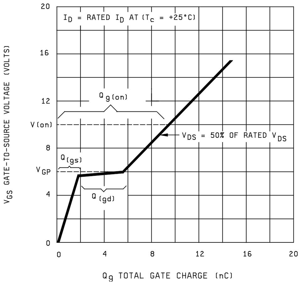
FIGURE 3471-4. Gate charge, condition B.
