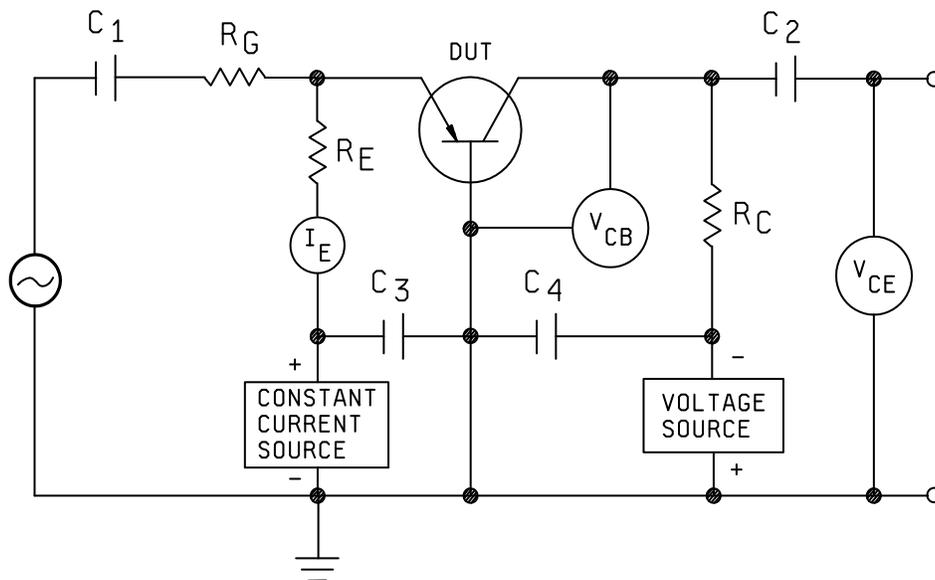
NOTE: Normal VHF circuit precautions should be taken. At frequencies higher than 10 MHz, the use of this circuit may lead to excessive errors. The biasing circuit shown is for the purposes of illustration only and any stable biasing circuit may be used.
