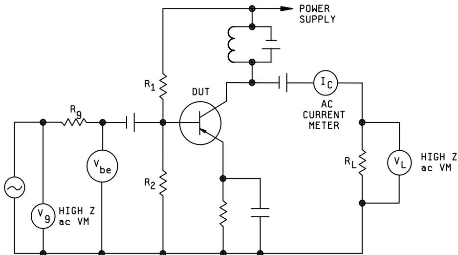
NOTE: For other configurations, the circuit should be modified in such a manner that the circuit is capable of demonstrating device conformance to the applicable specification sheet.
