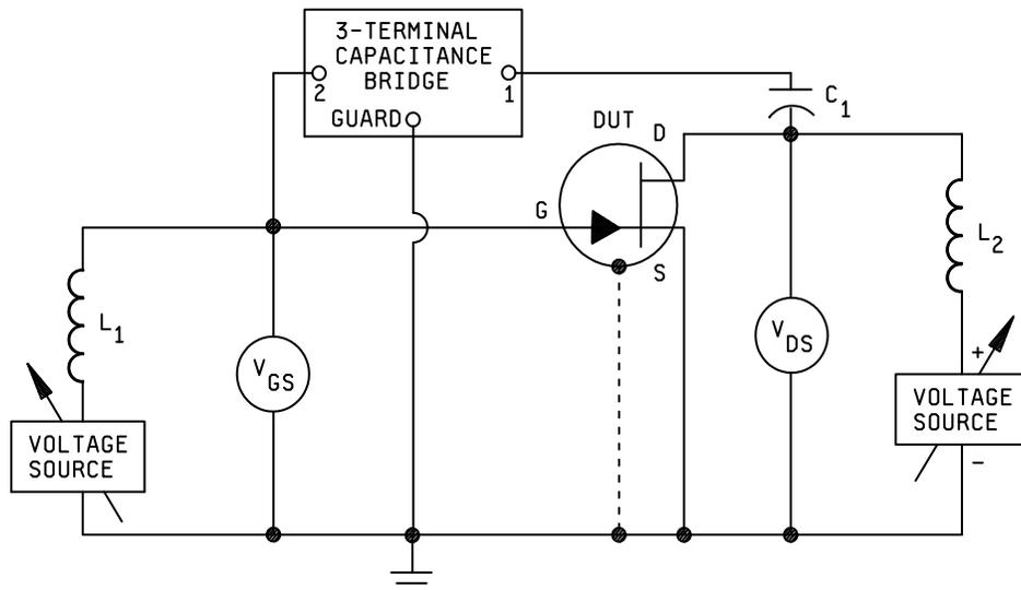
NOTE: The dotted connection between the case and ground shall be used for devices in which the case is not internally electrically connected to any element. If the case is internally electrically connected to any element, the dotted connection shall not be used.
