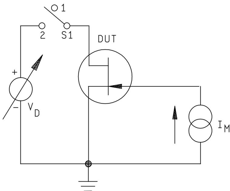
NOTE: The circuit consists of the DUT, one voltage source, one current source, and one electronic switch. During the heating phase of the measurement, switch S1 is in position 2. The value of  $V_D$  is adjusted to achieve the desired values of  $I_D$  and  $V_{DS}$  for the  $P_H$  heating condition.
