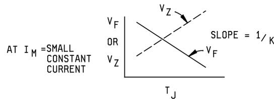
NOTE:  $I_M$  shall be large enough to overcome surface leakage effects but small enough not to cause significant self heating. When using the Zener direction, the  $I_M$  may also require adjustment to avoid a near zero TSP where the avalanche breakdown effects are offset by tunneling or field emission. (See 4.2.d.)
