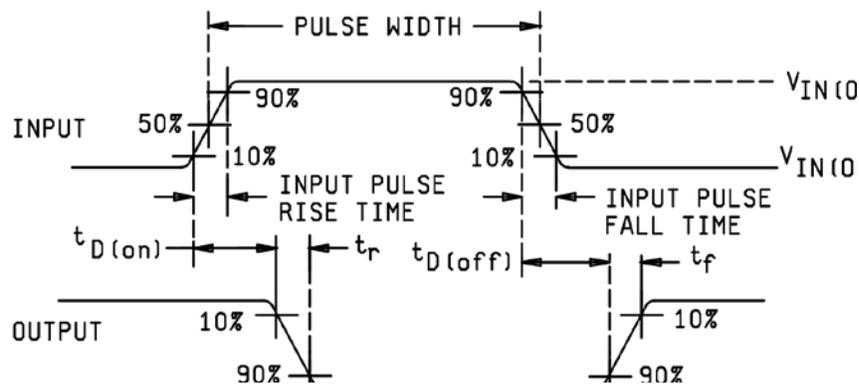
FIGURE 3459-1. Pulse characteristics.
