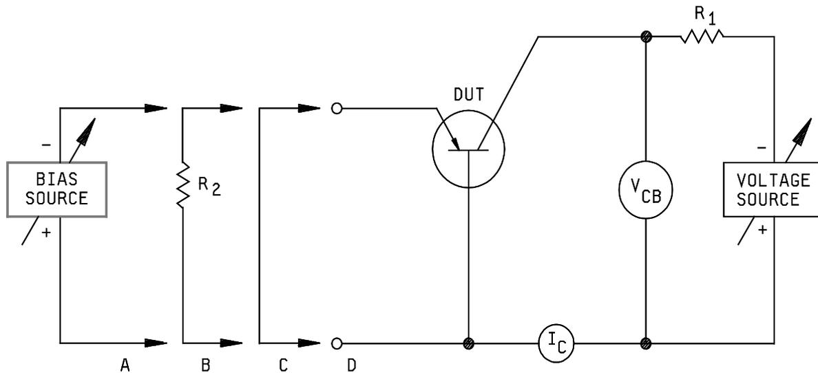
NOTE: The ammeter shall present essentially a short circuit to the terminals between which the current is being measured or the voltmeter readings shall be corrected for the ammeter drop.
