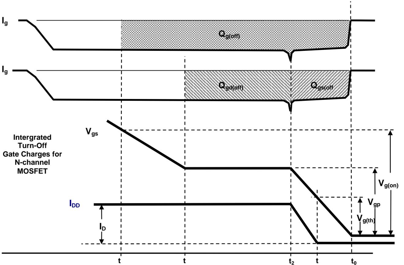
FIGURE 3471-7. Integrated Gate Charges, Condition B (turn-off).
