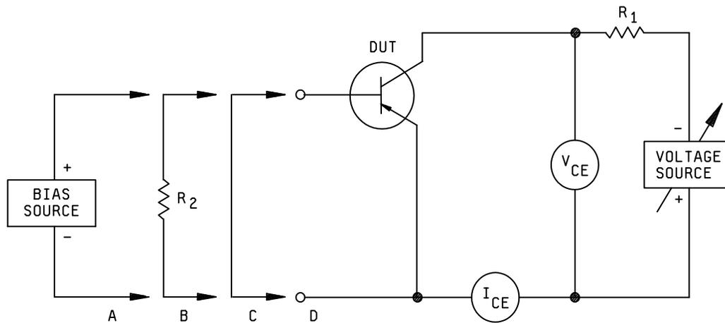
NOTE: The ammeter shall present essentially a short circuit to the terminals between which the current is being measured or the voltmeter shall be corrected for the drop across the ammeter.
