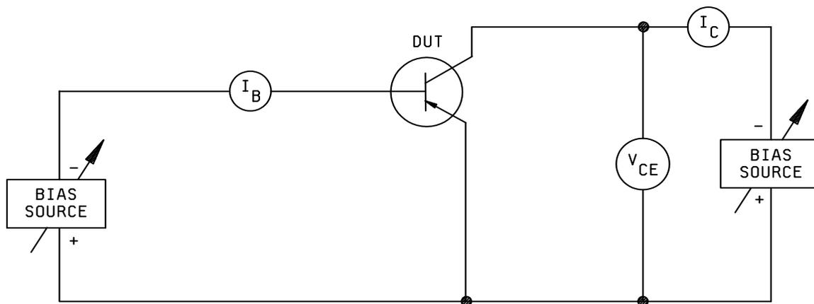
FIGURE 3030-1. Test circuit for collector to emitter voltage.
