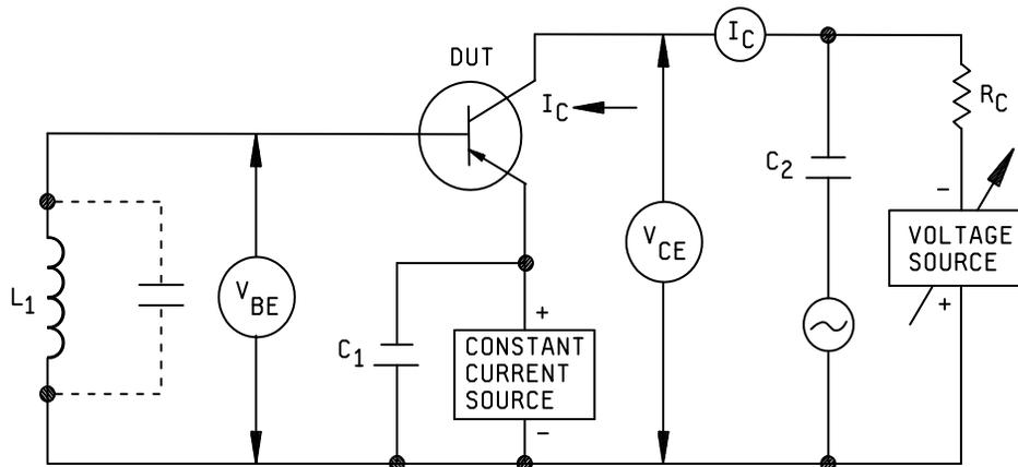
NOTE: The biasing circuit shown is for purposes of illustration only. Other stable biasing circuits may be used (see 3).
