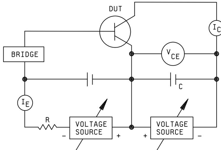
NOTE: The circuit shown is used for measuring the common emitter real part of the small-signal, short-circuit input impedance. For other device configurations, the above circuitry should be modified in such a manner that it is capable of demonstrating device conformance to the minimum requirements of the applicable specification sheet.
