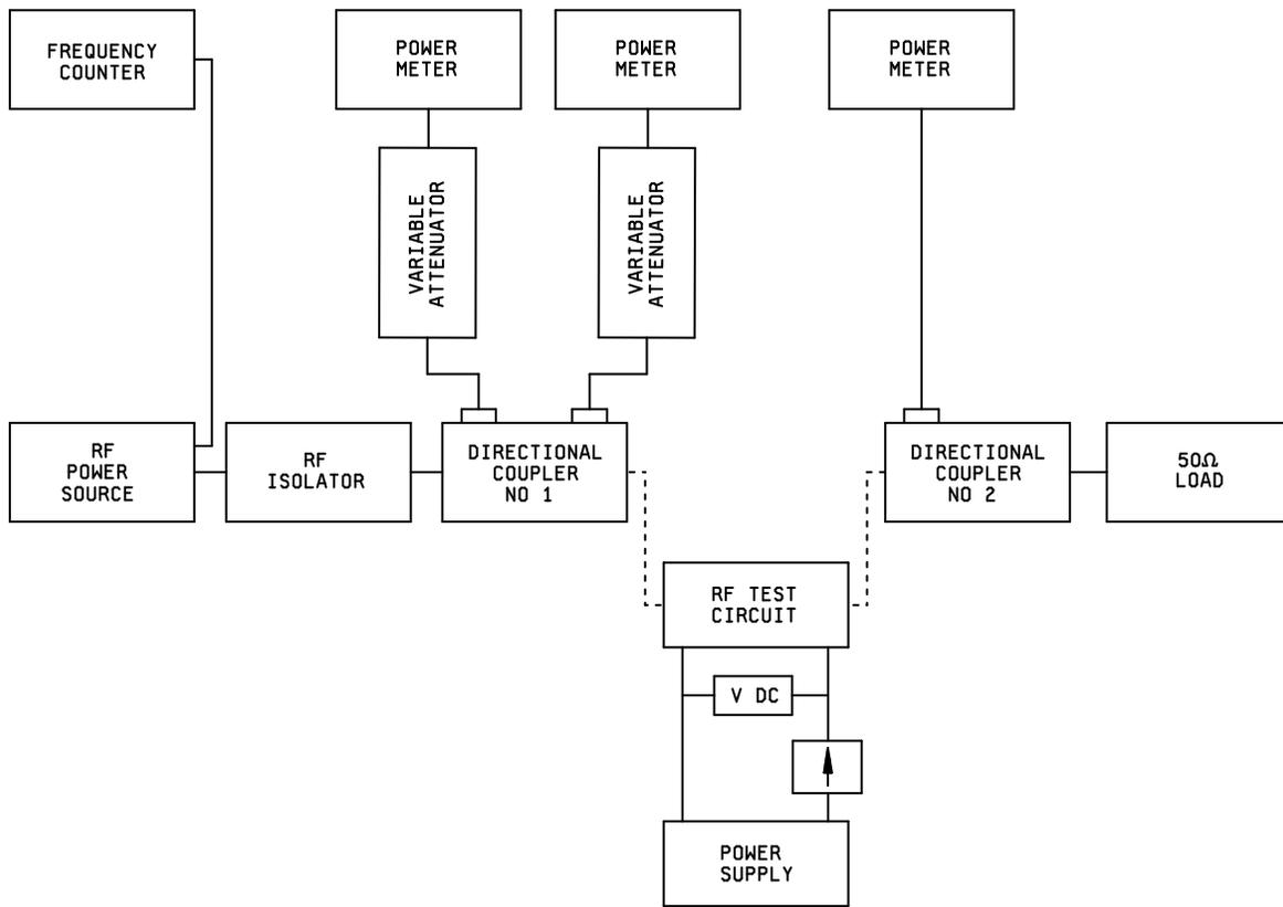
FIGURE 3320-3. RF test setup.
