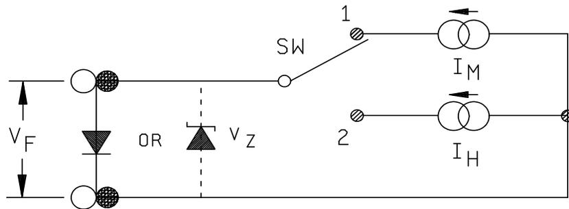
FIGURE 3101-1. Thermal impedance testing setup for diodes.
