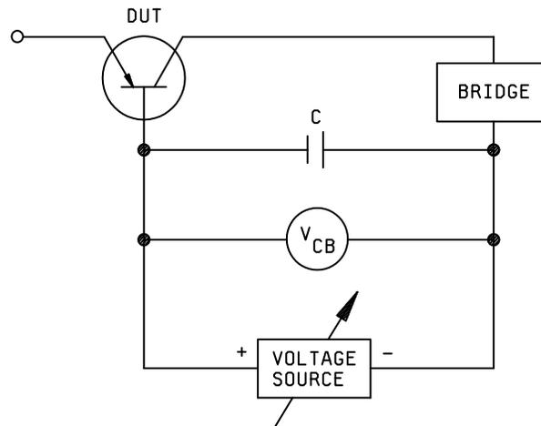
FIGURE 3236-1. Test circuit for open-circuit output capacitance.
