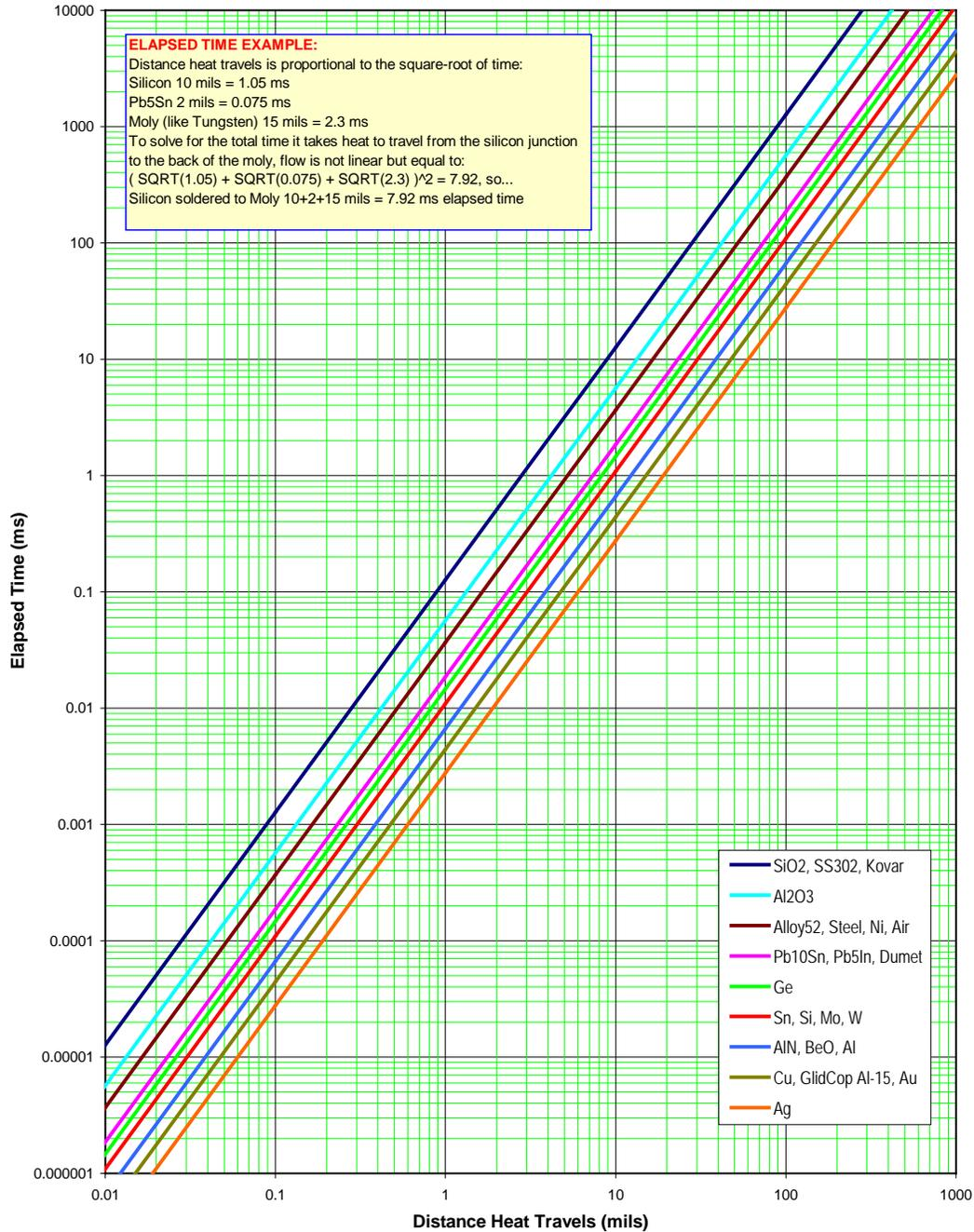
FIGURE 3101-A1 Heat flow distance vs. elapsed time plot.
