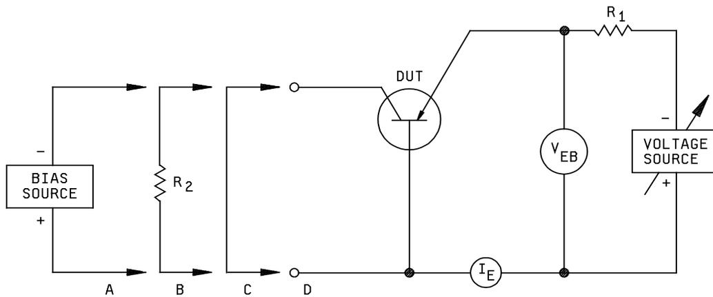
NOTE: The ammeter shall present essentially a short-circuit to the terminals between which the current is being measured or the voltmeter readings shall be corrected for the ammeter drop.
