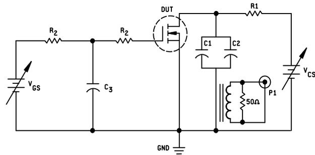
FIGURE 3478-1. Gate bias configuration 1.
