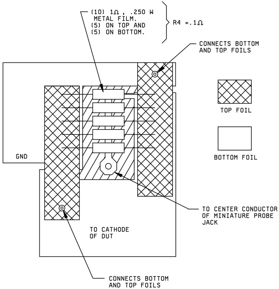
NOTE: Bottom resistor current flow is in opposite direction of top resistor current flow, providing magnetic field cancellation. Sense lead to center conductor of probe jack exits at right angle to resistor axes and is located between the resistor layers; five on the top layer and five on the bottom layer.
