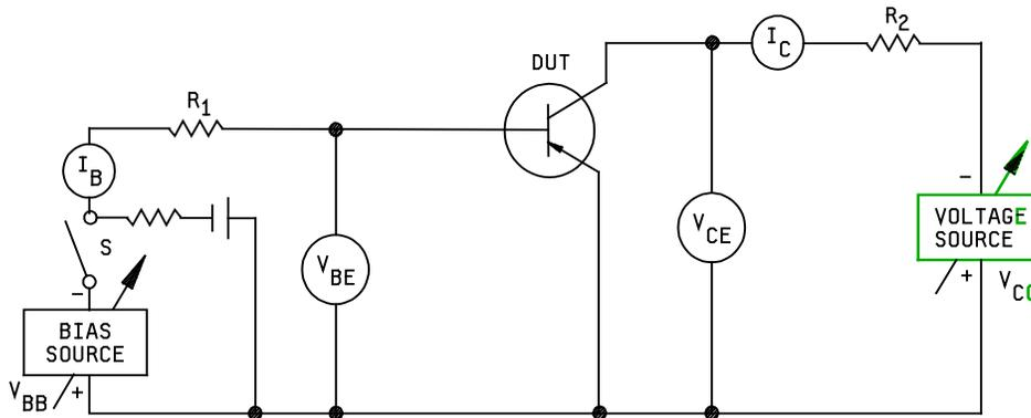
NOTE: If necessary, switch S shall be used to provide pulses of short duty cycle to minimize the rise in junction temperature. When pulsing techniques are used, oscillograph methods shall be used to measure  $V_{BE}$  and the other necessary parameters and the duty cycle and pulse width shall be specified.
