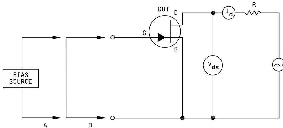
NOTE: The ac voltmeter shall have an input impedance high enough that halving it does not change the measured value within the required accuracy of the measurement.
