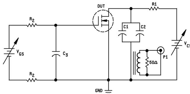
FIGURE 3478-2. Gate bias configuration 2.
