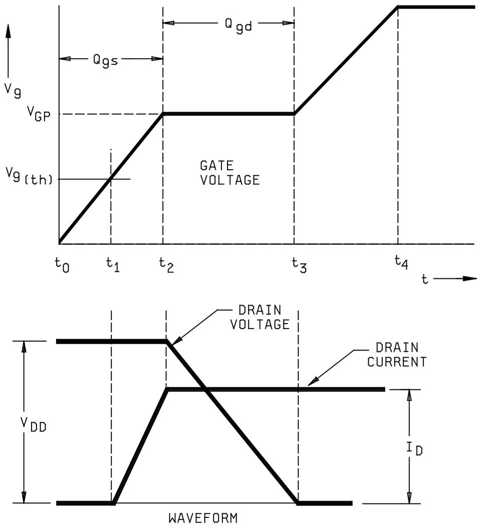
FIGURE 3471-5. Idealized gate charge waveforms, condition B.
