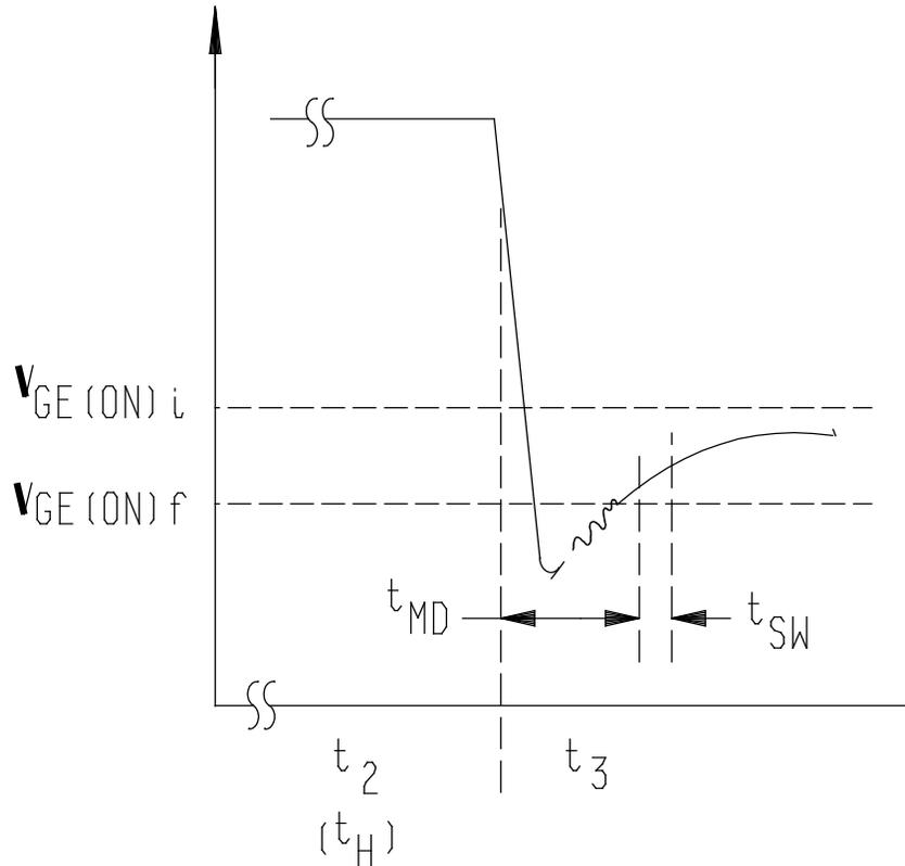
The value of  $t_{MD}$  is critical to the accuracy of the measurement and shall be properly specified in order to ensure measurement repeatability. Note that some test equipment manufacturers include the sample and hold window time  $t_{SW}$  within their  $t_{MD}$  specification.
