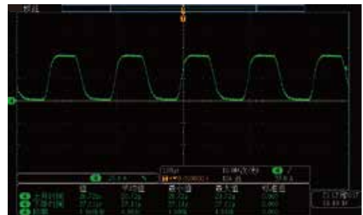
IT8906A-1200-240 5 kHz dynamic loading 0A-50A
