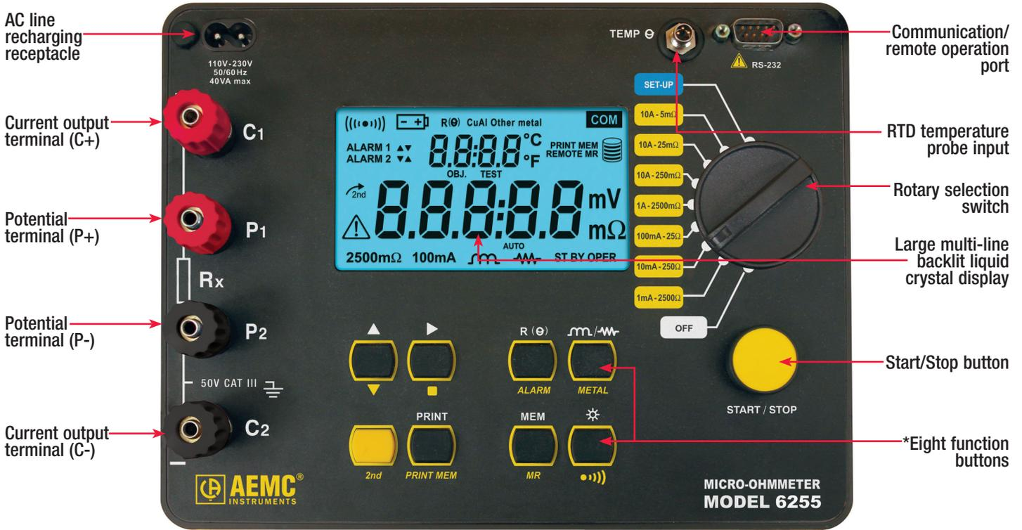
\* Function buttons allow direct access to data storage and retrieval, polarity reversal, auto/manual measurement and displayed values.
