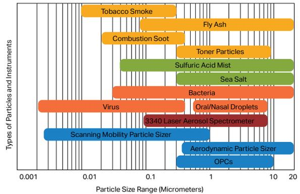
With a size range of 0.09 (90 nm) to 7.5 µm this is the right instrument to bridge the 1 µm particle size regime, measuring both the accumulation and course particle modes.
