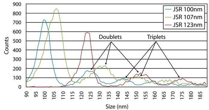
Typical resolution is within 2.5% of the particle diameter at 0.1 µm. The model 3340A can differentiate between 100 nm and 107 nm PSL!
