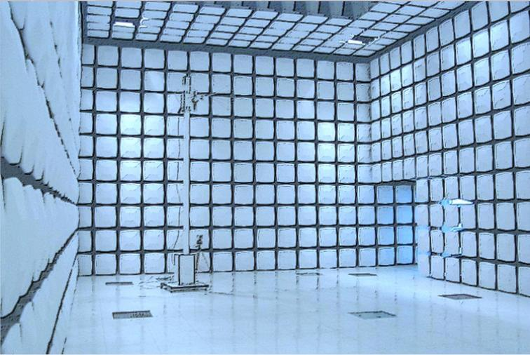
■ **SAC** (Semi-Anechoic Chamber) or **FAC** (Fully Anechoic Chamber)
