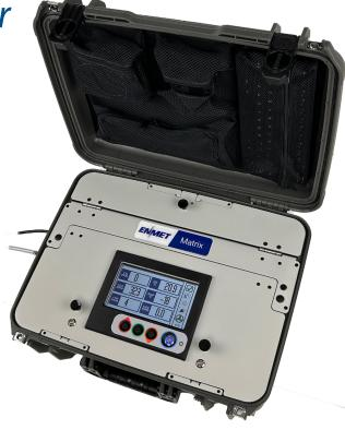
The MATRIX MedAir is designed to meet NFPA 99A and EN12021 requirements for analyzing and verification of medical and industrial breathing air sources.
