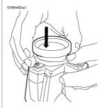
6 Rotate the lens 30° clockwise (looking at the front of the lens).
