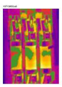
Figure 25.6 An isotherm in an infrared image of a fusebox
