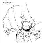
**5** Carefully push the lens cap into position.
