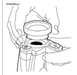
**5** Carefully push the lens into position.
