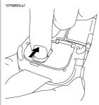
2 Open the cover to the battery compartment.
