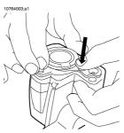
2 Rotate the lens cap 30° counter-clockwise (looking at the front of the lens).
