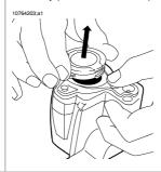
4 Correctly position the lens in front of the bayonet ring.
