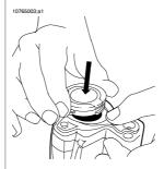
6 Rotate the lens cap 30° clockwise (looking at the front of the lens).
