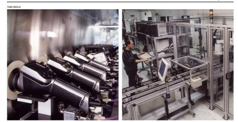
Figure 26.4 LEFT: Testing of infrared cameras in the climatic chamber; RIGHT: Robot used for camera testing and calibration
