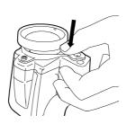
2 Rotate the lens counter-clockwise 30° (looking at the front of the lens).
