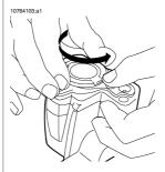
3 Carefully pull out the lens cap from the bayonet ring.
