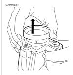
4 Correctly position the lens cap in front of the bayonet ring.
