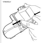
Push the rear part of the sunshield toward the screen, and then release your grip. Make sure that the two tabs mate with the corresponding notches.
