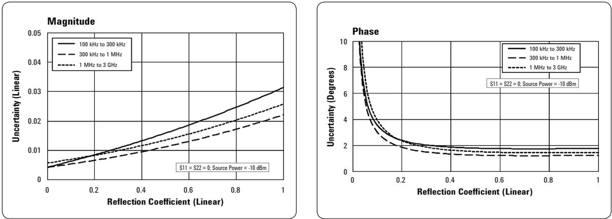
Table 7. Corrected system performance with Type-N 50 Ω connectors, 85092C ECal Module, full 2-port calibration
