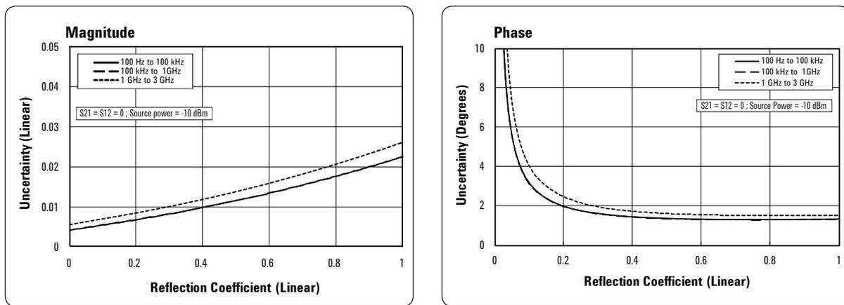
Table 4. Corrected system performance with Type-N 50 Ω connectors, 85092C ECal Module, full 2-port calibration
