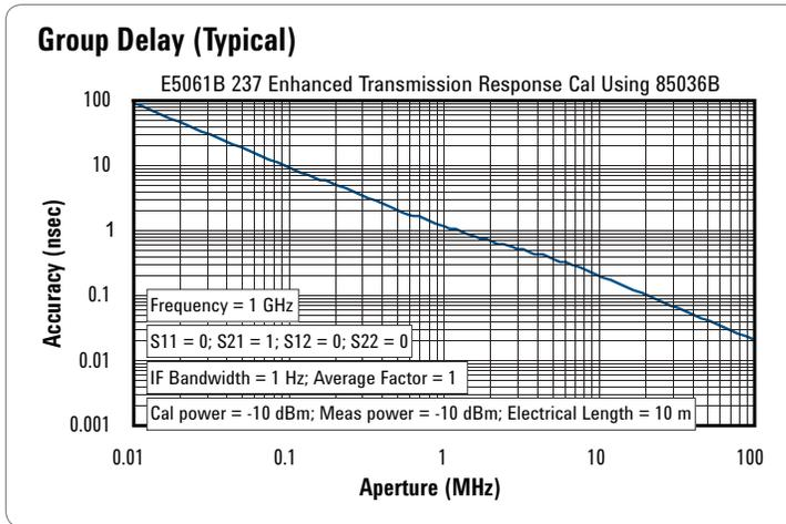
In general, the following formula can be used to determine the accuracy, in seconds, of specific group delay measurement:  $\pm \text{phase accuracy (deg)} / [360 \times \text{aperture (Hz)}]$
