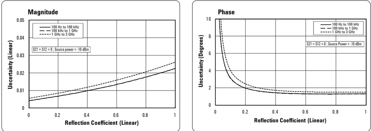
Table 3. Corrected system performance with Type-N 50 Ω connectors, 85032F calibration kit, enhanced response calibration
