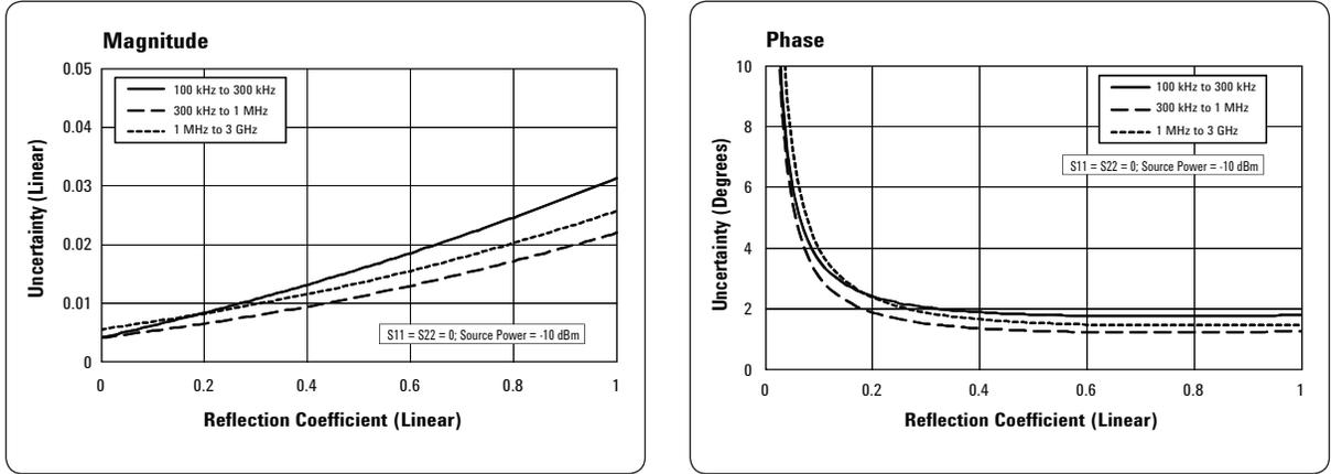
Table 6. Corrected system performance with Type-N 50 Ω connectors, 85032F calibration kit, enhanced response calibration
