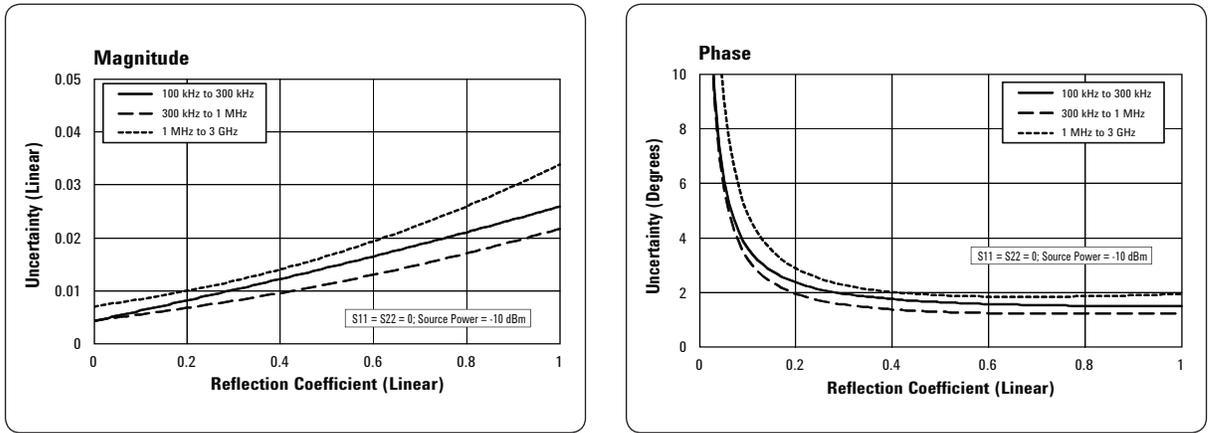
Table 9. Corrected system performance with Type-N 75 Ω connectors, 85036B calibration kit, enhanced response calibration
