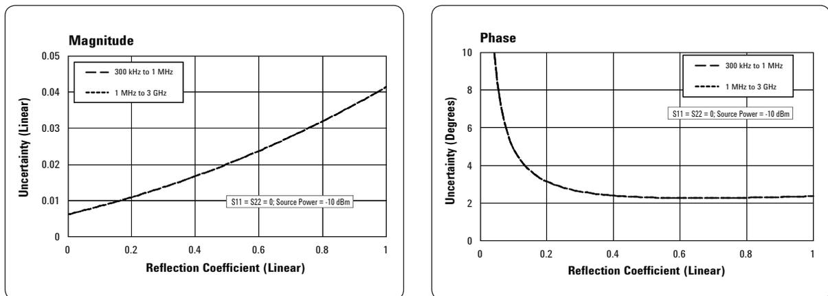
Table 8. Corrected system performance with Type-N 75 Ω connectors, 85036B calibration kit, full 2-port calibration
