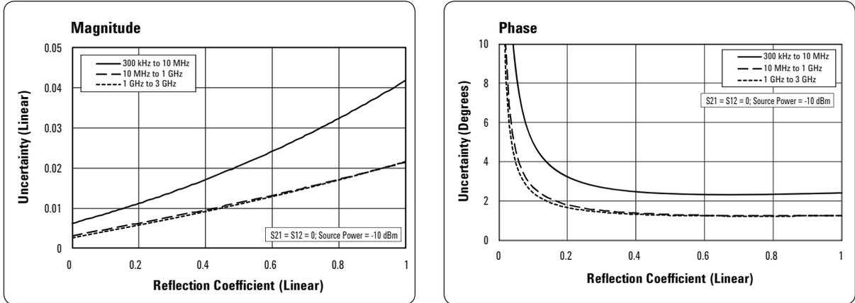
Table 5. Corrected system performance with Type-N 50 Ω connectors, 85032F calibration kit, full 2-port calibration
