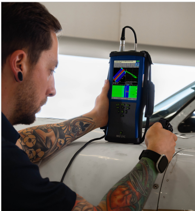
Figure 3: Axial encoder for bolt hole inspection.
