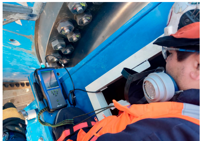
Figure 5: MIZ-21C performs conductivity and coating thickness measurement.
