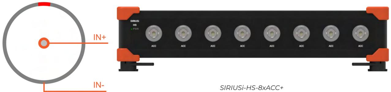
HS-ACC connector: pin-out (BNC)
