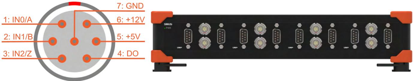
CNT connector: pin-out (7-pin LEMO female)
