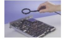
■ real burst with changing amplitude and frequency EFT's are injected using the integrated single phase CDN, capacitive coupling clamp external three phase CDN or direct into electronic circuits using the electric and magnetic field generation probes.
