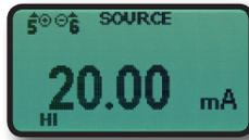
Source & Read 0.00 to 24.00 mA, Simulate a 2 Wire Transmitter or use the PIECAL 820 to simultaneously power your 2 Wire Transmitter and measure its output.
