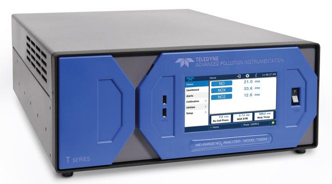
The Model T200M Mid-Range NO / NO $_2$  /NO $_3$  analyzer uses the proven chemiluminescence detection principle and advanced electronics to allow accurate, dependable, continuous measurements for mid-level stack gas monitoring and other applications. The T200M may be fitted with an optional, internal paramagnetic O $_2$  sensor or an infrared absorption CO $_2$  sensor, reducing integration and operating costs significantly.
